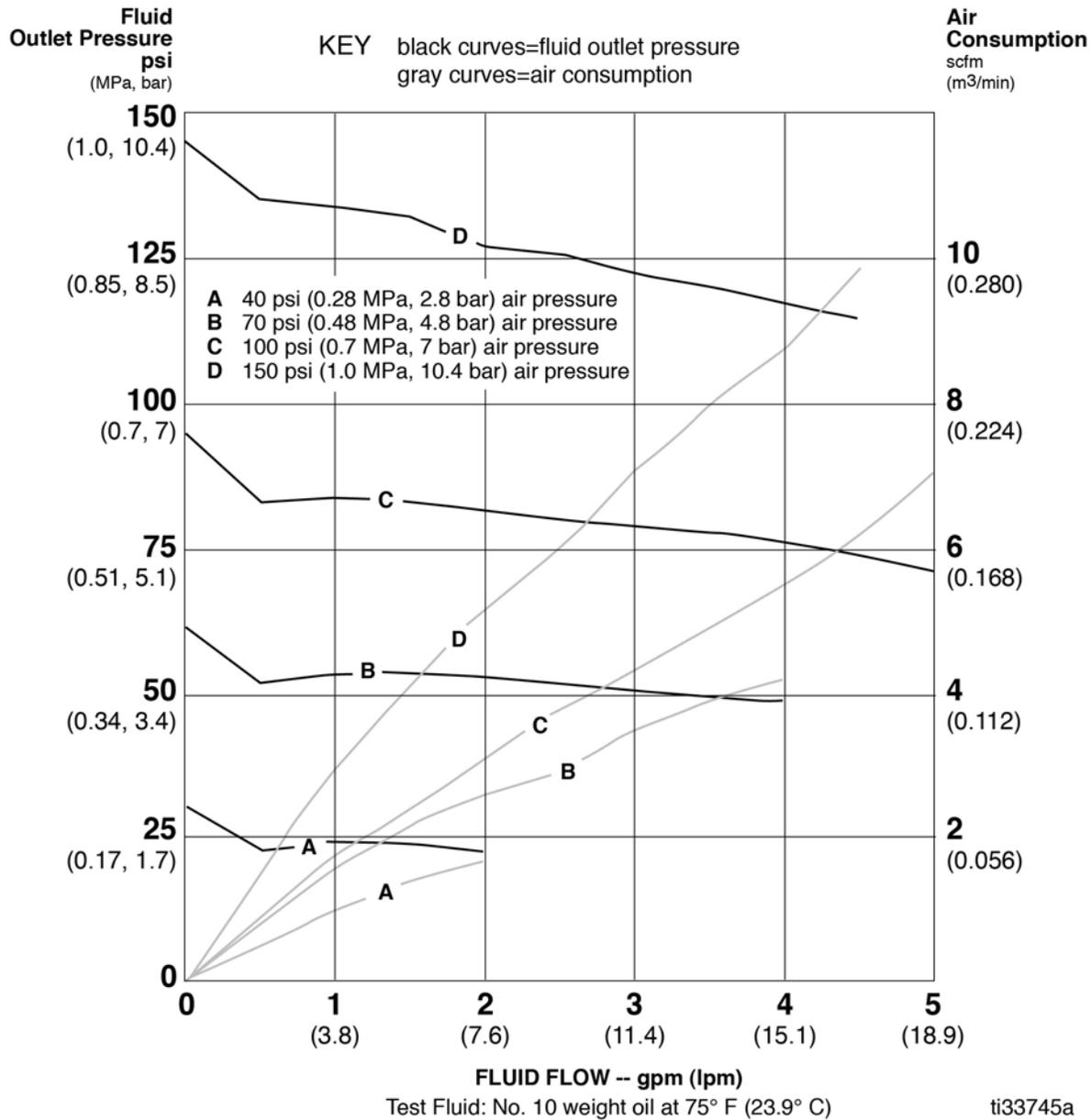
**To find fluid outlet pressure** at a specific fluid flow and operating air pressure:
