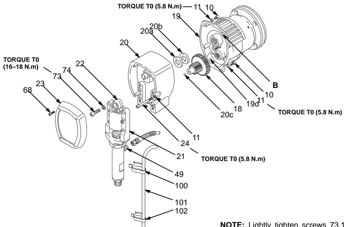
**NOTE:** Lightly tighten screws 73,10 and 24 oppositely and evenly. Then tighten oppositely and evenly again to the specified torque.
