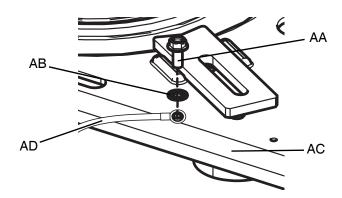
Fig. 2: Grounding Connection on Pump
