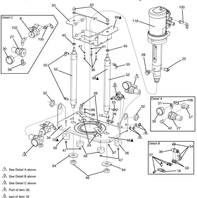
Fig. 8: DynaMite 190 Extruder Assembly Parts without Air Tubing
