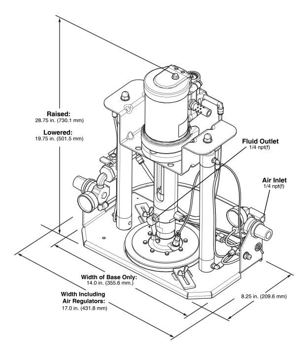
Fig. 15: DynaMite 190 Extruder Assembly Dimensions
