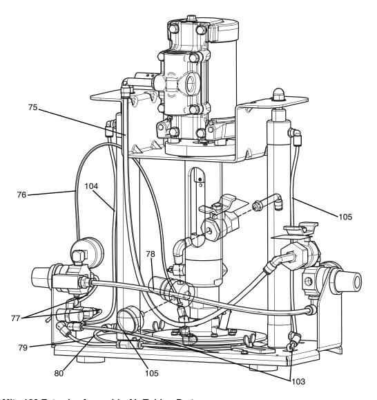
Fig. 9: DynaMite 190 Extruder Assembly Air Tubing Parts
