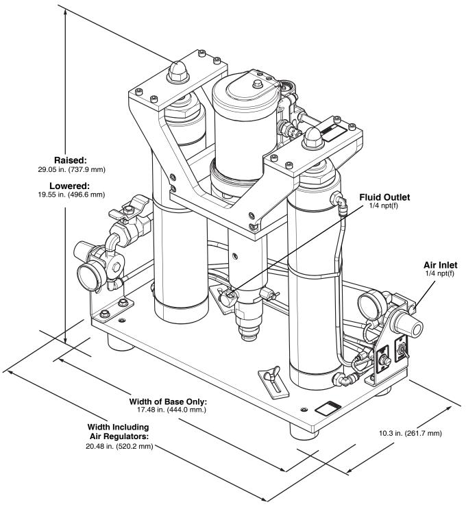
Fig. 16: DynaMite 190 Extruder Assembly Dimensions
