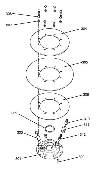
Fig. 14: Wiper Plate Parts
