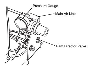
Fig. 3: Pressure Relief Components
