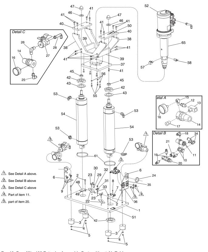
Fig. 10: DynaMite 190 Extruder Assembly Parts without Air Tubing
