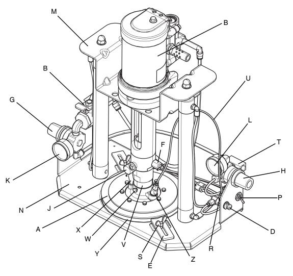
Fig. 1: System Components
