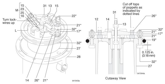
FIG. 4 Air Motor and Throat
