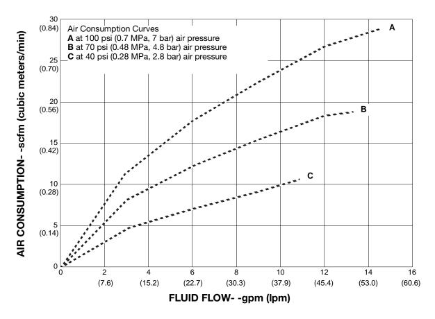
To find Pump Air Consumption (sctm or m#/min) at a specific fluid flow (gpm/lpm) and air pressure (psi/MPa/bar):
