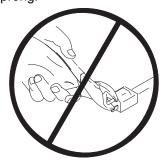
Only use an **extension cord** with an undamaged 3-prong plug. Recommended extension cords for use with this sprayer:
