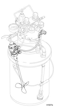
Agitator Kit shown installed on TRITON 308 spray package (not included)
