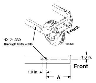
A = 6.55 in. — LineLazer 3500 & 5000 (must be drilled)
