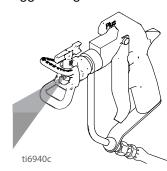
5. Hold the gun perpendicular and approximately 12 in. (30 cm) from the surface. Move the gun first, then pull the gun trigger to spray.
