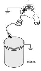
**Maintain Grounding Continuity:** When flushing or relieving pressure, hold a metal part of the gun firmly against the side of a grounded metal pail, then trigger the gun.
