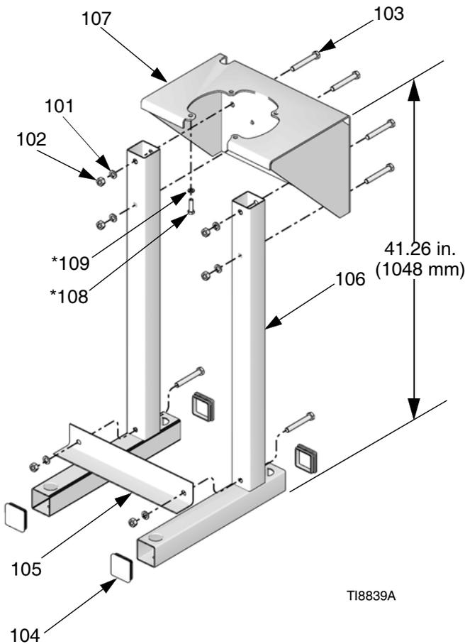
**NOTE:** Adapter plate 247312 is required to mount an NXT 2200 air motor to the bracket. Order separately.
