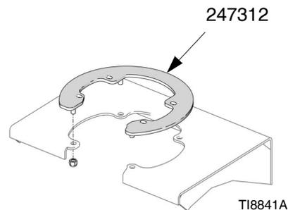
4. Drill four 7/16 in. (11 mm) holes using the bracket as a template. Use hole groups P1 or P2. (See **Wall Bracket Mounting Hole Diagram**, page 2.)
