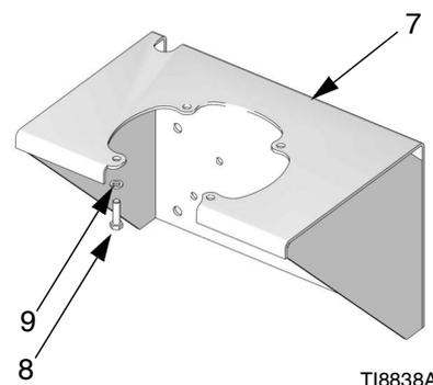
**NOTE:** Adapter plate 247312 is required to mount an NXT 2200 air motor to the bracket. Order separately.
