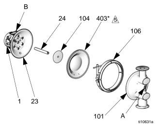
Apply medium strength (blue) Loctite® or equivalent to bolt (not shown).
