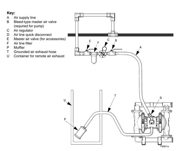
Fig. 4 Venting Exhaust Air
