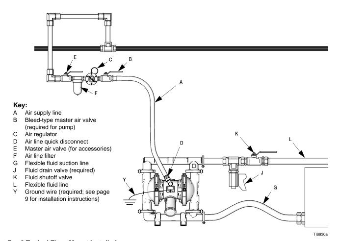
Fig. 2 Typical Floor-Mount Installation
