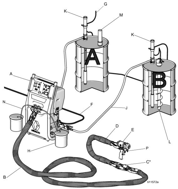
\* Shown exposed for clarity. Wrap with tape during operation.
