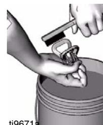
19. Wipe paint off outside of gun using a soft cloth moistened with water or flushing solvent.
