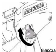
14. Stop triggering gun. Engage trigger lock.
