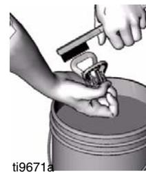
24. Wipe paint off outside of gun using a soft cloth moistened with water or flushing solvent.
