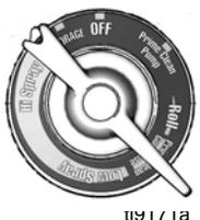
e. Continue to hold gun trigger until you see paint diluted with flushing fluid starting to come out of gun.
