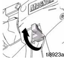
2. Verify tip and guard parts are assembled in order as shown below.
