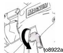
5. When obstruction is cleared, lock trigger lock and rotate arrow-shaped handle back to SPRAY position.
