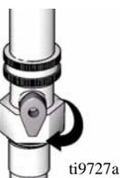
8. Turn lever to close power flush attachment.
