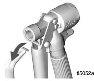
3. The trigger guard beneath the gun handle can then be used as a wrench to loosen the nut.
