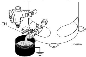
13. Close the material drain (EH) and fill the hopper with solvent.
