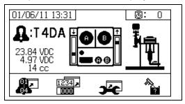
There are two levels of alarms: warnings and advisories. A bell icon indicates an alarm. A solid bell icon with an exclamation point and three audible alerts indicate a warning. And an outlined hollow bell icon and a single audible alert indicate an advisory.
