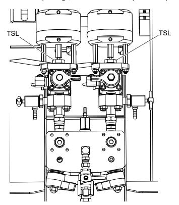
For pump and dosing valves, check packing nut tightness after first hour of operation and again after 24 hours. Then check when TSL discolors or seeps over packing nut. Also check tightness whenever sprayer is transported. Tighten packing nuts only when all fluid pres.ure is relieved. Continue to follow maintenance procedure intervals regarding all seals, page 64.
