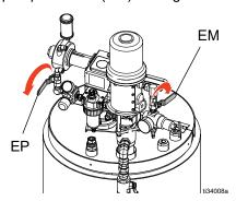
11. Run the main high pressure fluid pumps until the material has been emptied out of the system, press
