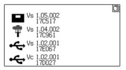
This screen displays the versions and part number of the system components. Refer to the following table for details. To access this screen, press from the Home Setup screen.
