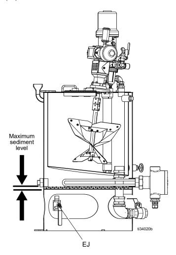
**NOTE:** The immersion heater will not operate in sediment deposits.
