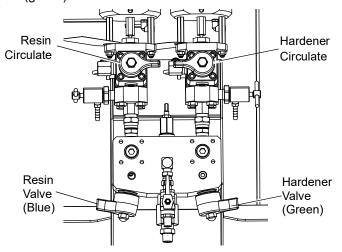
3. Adjust pump air regulator to 30 psi (0.21 MPa, 2.1 bar).
