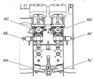
Place a clean container under sampling valve A (AE).
