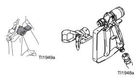
Disengage trigger lock and trigger gun into a grounded pail. Use a pail lid with a hole to dispense through. Seal around hole and gun with a rag to prevent splash back. Be careful to keep fingers away from front of gun.
