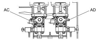
4. When each blue pump LED turns off, close the corresponding circulation valve.
