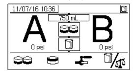
If the system ratio mode is by volume, either volumes or weights can be measured.
