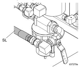
Air supply requirement: 150 psi (1.0 MPa, 10.3 bar) maximum; 50 psi (0.35 MPa, 3.5 bar) minimum while running **System Verification** (page 51), and 80 psi (0.55 MPa, 5.5 bar) while spraying.
