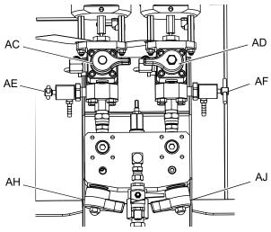
b. Place a clean 1 quart (1000 cc) container under sampling valve A (AE).
