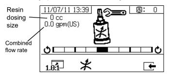
The restrictor adjust bar graph is shown when \* is pressed. This screen is used to adjust the restrictor.
