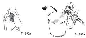
6. Open solvent pump air valve (CB). Pull out and slowly turn solvent pump air regulator (CG) clockwise to prime solvent pump and push air out of mix hose and gun. Trigger gun until all air is purged.
