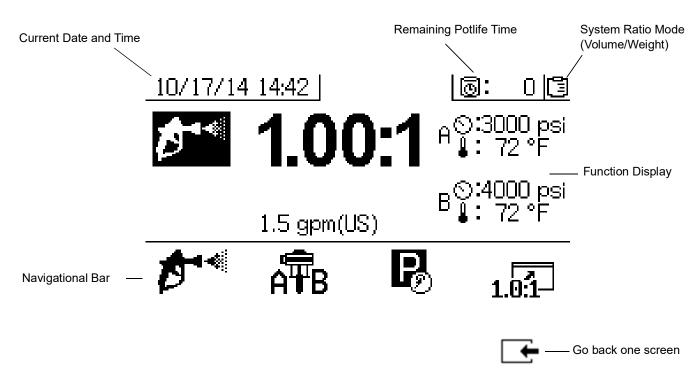
Fig. 6: Main Display Screen Components (shown with all display features enabled)
