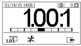
The ratio bar graph is shown when 1 is pressed. This screen is used to show the accuracy of the spray ratio. The bar should be in the center three segments when the restrictor is adjusted.
