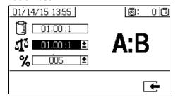
For Ratio by Volume Mode, use this screen to set the ratio by weight (middle number), and the ratio tolerance (bottom number). The values determine whether the ratio test passes. The ratio by volume (top number) is displayed but cannot be changed on this screen. Follow
