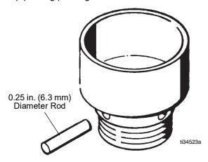
Adjust the packing nut weekly so it is just tight enough to prevent leakage. Use a spanner wrench or a 0.25 in. (6.3 mm) diameter rod to tighten the nut. Do not over-tighten. Never leave the pump or hoses filled with water or air. To help prevent corrosion, flush the water and all air out of the system and leave it filed with mineral spirits or an oil-based solvent.
