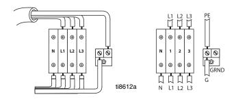
**380V, 3 Phase WYE:** Use a screwdriver to connect three power leads to the top terminals L1, L2, and L3. Connect neutral to N. Connect green to ground (GND).
