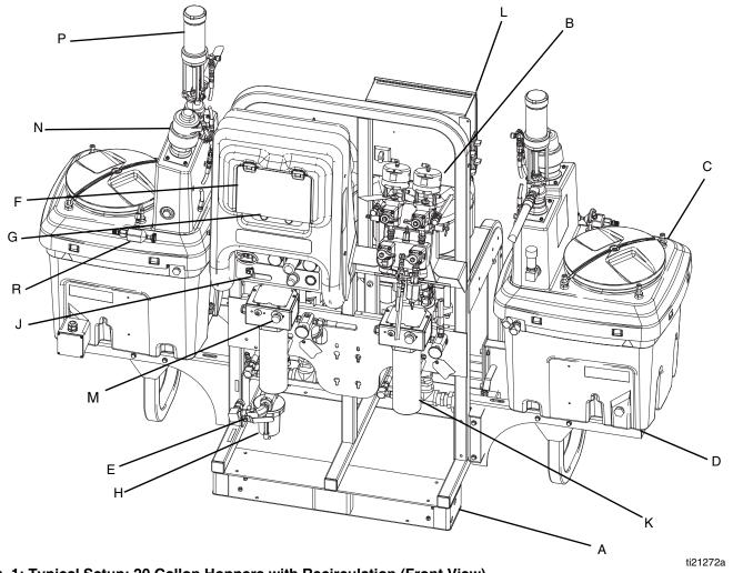
Fig. 1: Typical Setup: 20 Gallon Hoppers with Recirculation (Front View)
