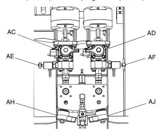
Place a clean container under sampling valve A (AE).
