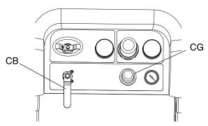
7. Close solvent pump air valve (CB) and trigger gun to relieve pressure. Engage gun trigger lock.
