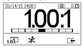
The ratio bar graph is shown when 101 is pressed. This screen is used to show the accuracy of the spray ratio. The bar should be in the center three segments when the restrictor is adjusted.
