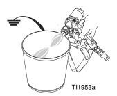
Engage trigger lock, turn off air regulator, and close main air shutoff valve. Remove spray tip.
