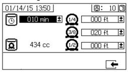
This screen enables users to set the potlife timer, and length of each mixed material hose specific to the system. The total mixed material volume is then calculated and displayed on the page. The potlife time displays in the upper right corner.
