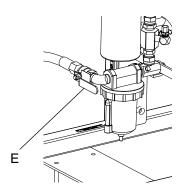
Air supply requirement: 150 psi (1.0 MPa, 10.3 bar) maximum; 50 psi (0.35 MPa, 3.5 bar) minimum (while running).
