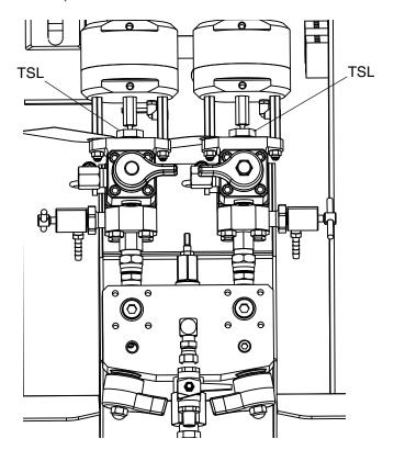
For pump and meter valves, check packing nut tightness after first hour of operation and again after 24 hours. Then check as needed, or when TSL discolors or seeps over packing nut. Also check tightness whenever sprayer is transported. Tighten packing nuts only when all fluid pressure is relieved.
