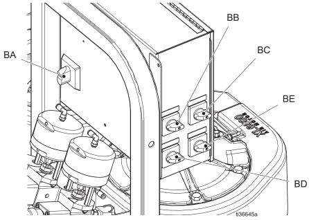
Fig. 4: Junction Box/Heater Controls
