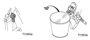
Open solvent pump air valve (CB). Pull out and slowly turn solvent pump air regulator (CG) clockwise to prime solvent pump and push air out of mix hose and gun. Trigger gun until all air is purged.
