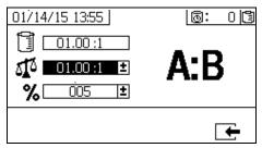
For **Ratio by Volume Mode**, use this screen to set the ratio by weight (middle number), and the ratio tolerance (bottom number). The values determine whether the ratio test passes. The ratio by volume (top number) is displayed but cannot be changed on this screen. See **Home** screen, on page 55, to change the ratio by volume.
