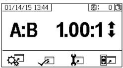
Home is the first screen that displays in Setup mode. It shows the current metering pump ratio and enables users to change the mix ratio and access the following screens: system setup, enable/disable functions, maintenance setup, and limits. Refer to the following table for more details.
