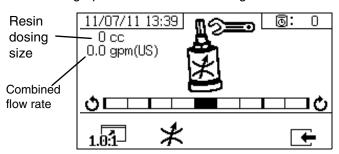
The restrictor adjust bar graph is shown when  $\bigstar$  is pressed. This screen is used to adjust the restrictor.
