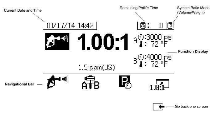
Fig. 7: Main Display Screen Components (shown with all display features enabled)
