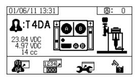
There are two levels of error codes: alarms and advisories. A bell icon indicates an alarm. A solid bell icon with an exclamation point and three audible alerts indicate a alarm. And an outlined hollow bell icon and a single audible alert indicate an advisory.
