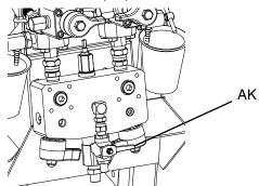
16. Release any residual gun pressure and engage trigger lock.
