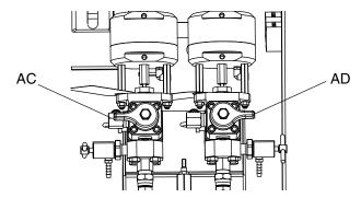
4. When each blue pump LED turns off, close the corresponding circulation valve.
