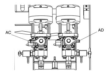
When priming or flushing the pumps, it is normal to get cavitation or pump runaway alarms. Clear the alarms
