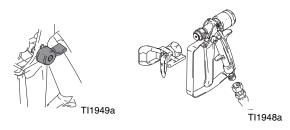
Disengage trigger lock and trigger gun into a grounded pail. Use a pail lid with a hole to dispense through. Seal around hole and gun with a rag to prevent splash back. Be careful to keep fingers away from front of gun.
