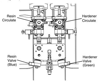
3. Adjust pump air regulator to 30 psi (0.21 MPa, 2.1 bar).
