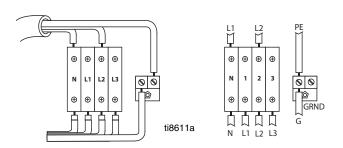
**230V, 3 Phase Delta:** Use a screwdriver to connect three power leads to top terminals L1, L2, and L3. Connect green to ground (GND).
