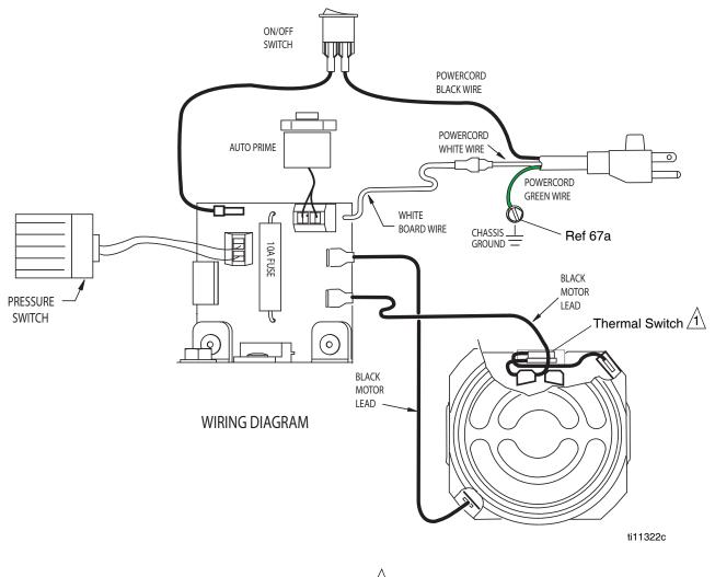
(1) When assembling motor to pump housing, make sure Thermal Switch is positioned on top as shown above.
