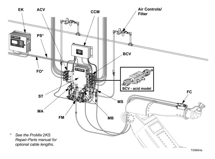
Fig. 3. Wall Mount System, shown with G3000 Meters, Color/Catalyst Change, Accessory Solvent Meter, and Flow Control
