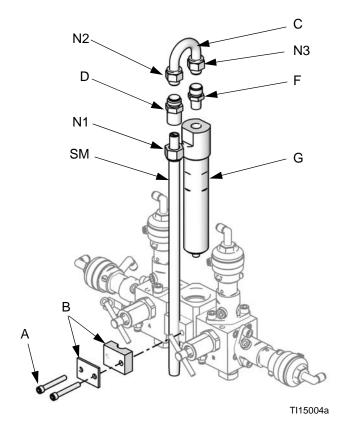
Fig. 12. Disassemble Integrator and Static Mixer
