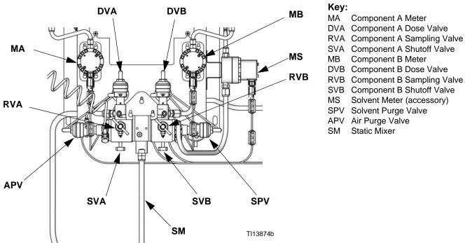
Fig. 14. Wall Mount Fluid Station, Dynamic Dosing
