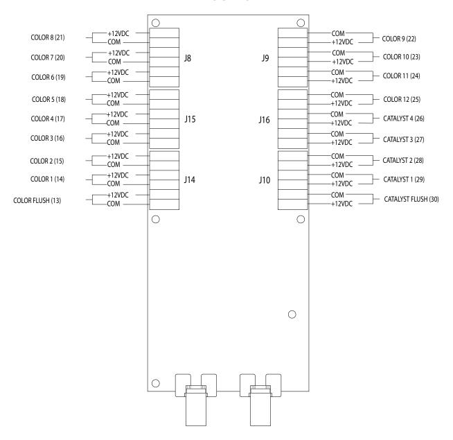
Fig. 22. Color Change Module Electrical Schematic
