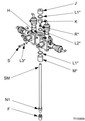
Fig. 13. Install 15U955 Injection Kit
