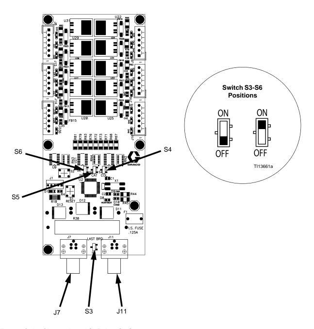
Fig. 21. Color Change Board Switches S3-S6
