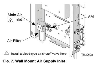
Install a bleed-type air shutoff valve here.
