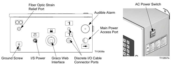
Fig. 18. EasyKey Connections and AC Power Switch
