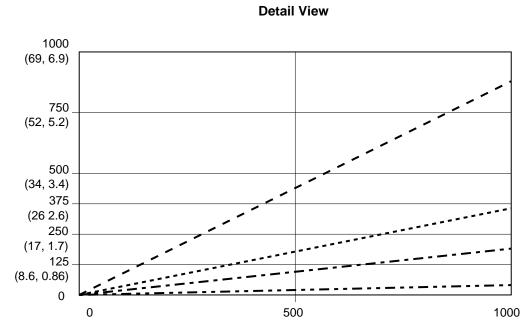
Fig. 28. Dynamic Dosing Performance (1:1 Ratio, 90 centipoise fluid, 100 psi A side pressure)
