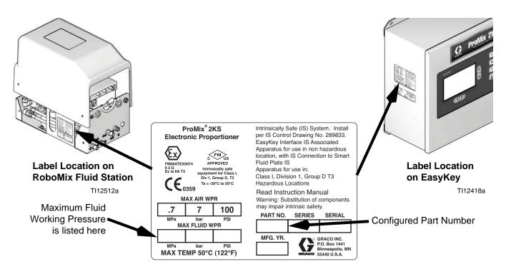
Fig. 2: Identification Label, RoboMix Fluid Station Systems
