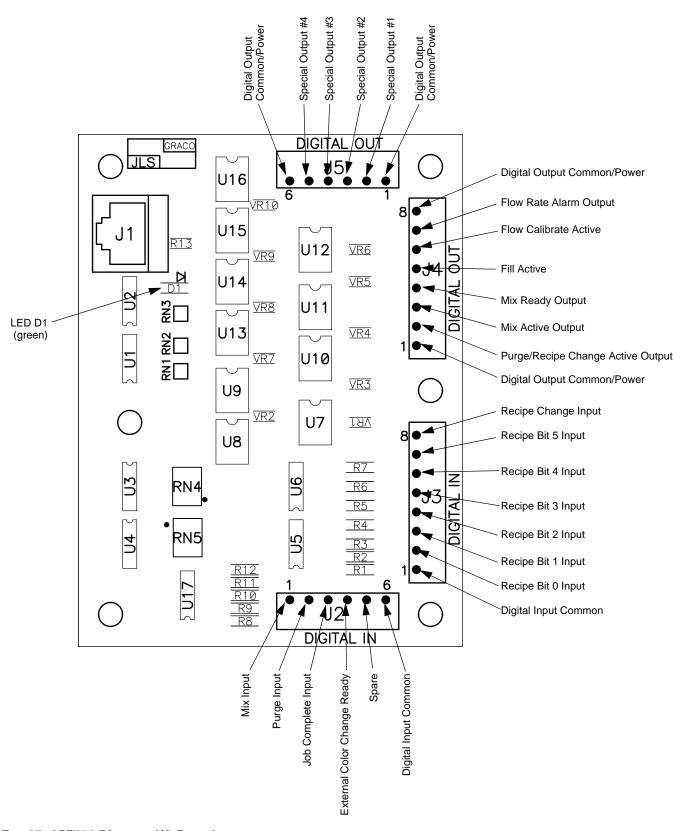
Fig. 27: 255766 Discrete I/O Board
