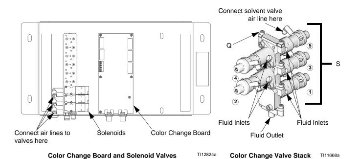
Fig. 11. Color Change Valves Air and Fluid Connections
