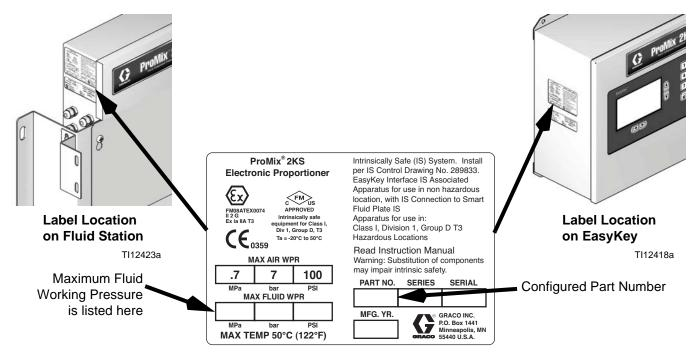
Fig. 1: Identification Label, Wall Mount Fluid Station Systems
