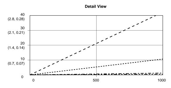
Fig. 32. Dynamic Dosing Performance (30:1 Ratio, 90 centipoise fluid, 100 psi A side pressure)
