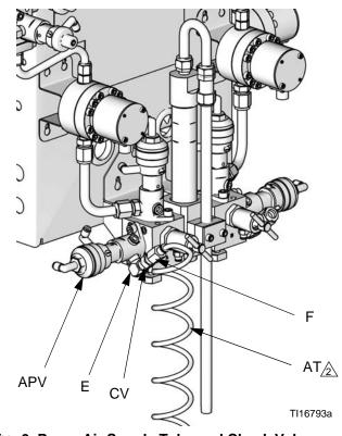
Fig. 9. Purge Air Supply Tube and Check Valve
