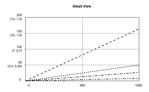
Fig. 30. Dynamic Dosing Performance (10:1 Ratio, 90 centipoise fluid, 100 psi A side pressure)
