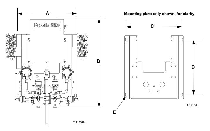
**NOTE:** Height is shown from top of panel to fluid shutoff valves, and does not include the effect of variable fluid integrator heights. Width of panel does not include optional color/catalyst valve stacks.
