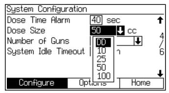
Fig. 32. Configure Screen 4, dynamic dosing selected
