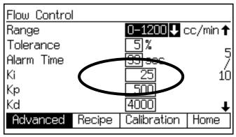
Fig. 101. Advanced Setup Screen 5 (Automatic Mode with Flow Control Only)
