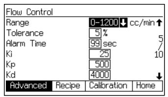
Fig. 44. Advanced Setup Screen 5 (Automatic Mode with Flow Control Only)
