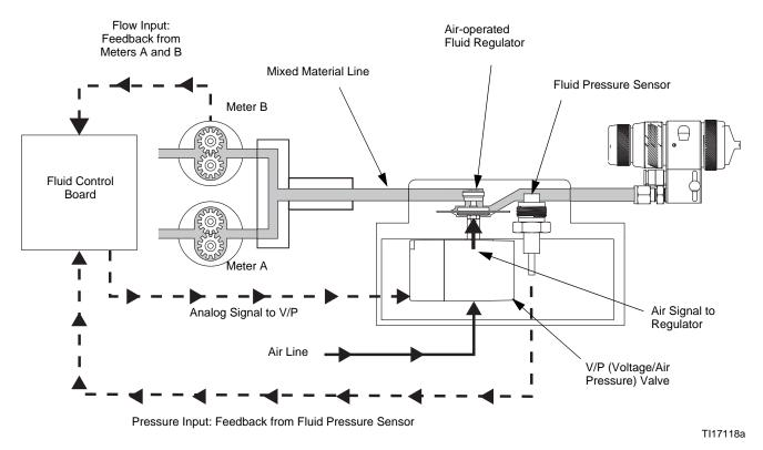
Fig. 86. ProMix Flow Control Schematic Diagram (249849 Module)
