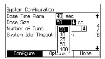
Fig. 107. Configure Screen 4, dynamic dosing selected
