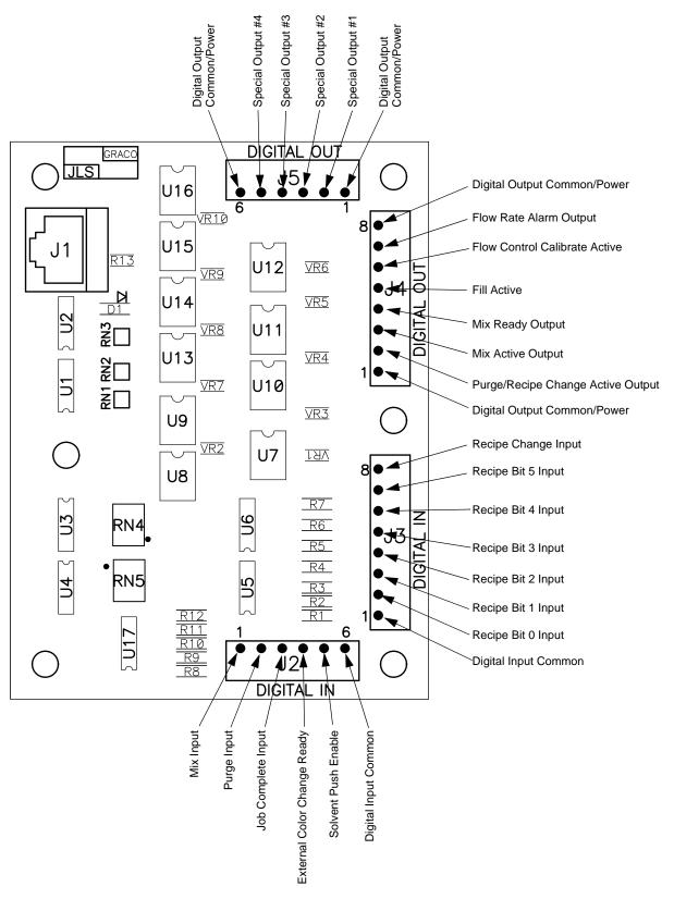
Fig. 70: 255766 Discrete I/O Board
