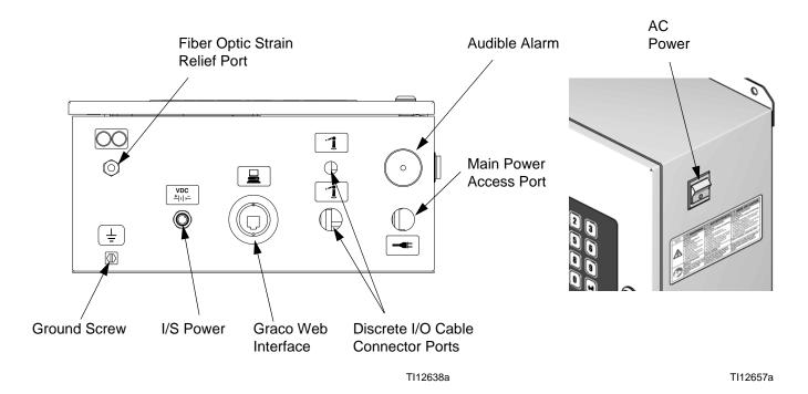
Fig. 8. EasyKey Connections and AC Power Switch
