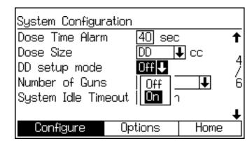
Fig. 108. Configure Screen 4, dynamic dosing setup mode enabled
