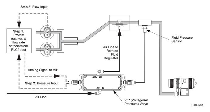
Fig. 89. ProMix Flow Control Pressure Loop and Flow Loop (24H989 Module)
