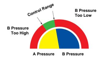
Fig. 110. A/B Control Range with Properly Sized Restrictor
