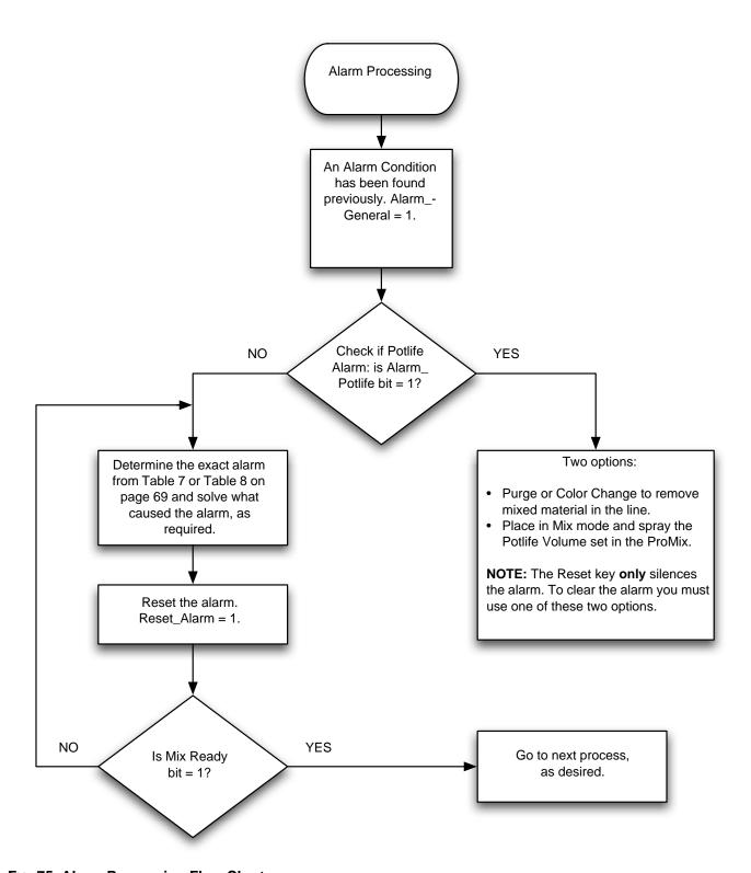
Fig. 75. Alarm Processing Flow Chart
