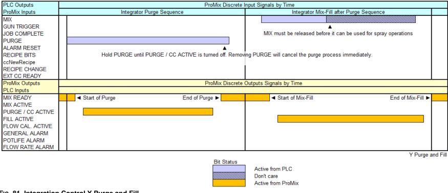
Fig. 81. Integration Control Y Purge and Fill
