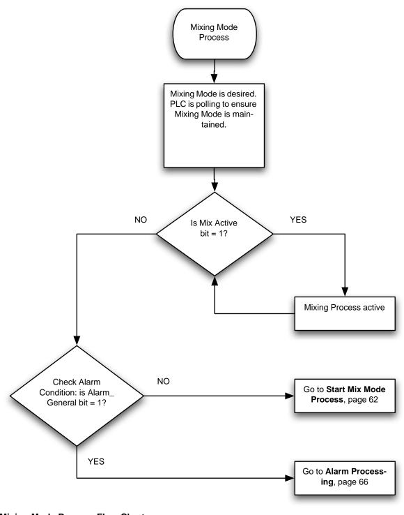
Fig. 72. Mixing Mode Process Flow Chart
