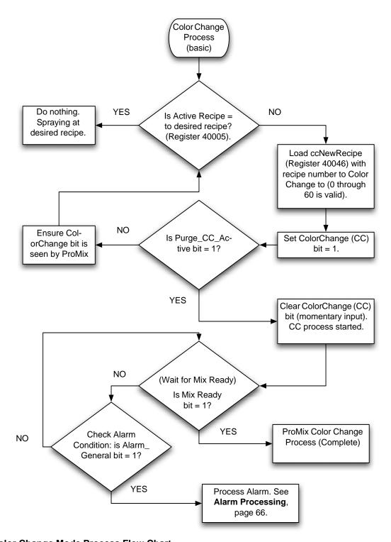
Fig. 74. Color Change Mode Process Flow Chart
