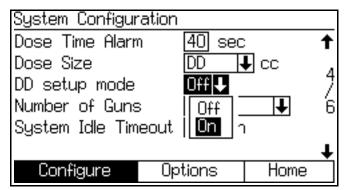
Fig. 33. Configure Screen 4, dynamic dosing setup mode enabled
