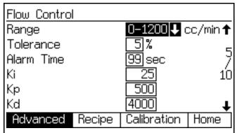
Fig. 95. Advanced Setup Screen 5 (Automatic Mode with Flow Control Only)
