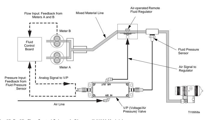
Fig. 87. ProMix Flow Control Schematic Diagram (24H989 Module)
