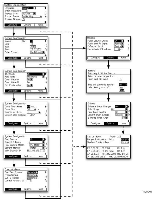
Fig. 27. System Configuration and Option Screens Map
