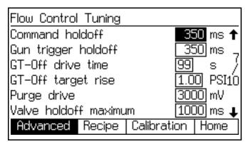
Fig. 46. Advanced Setup Screen 7
