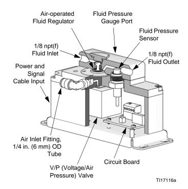
Fig. 84. Cutaway of 249849 Flow Control Module
