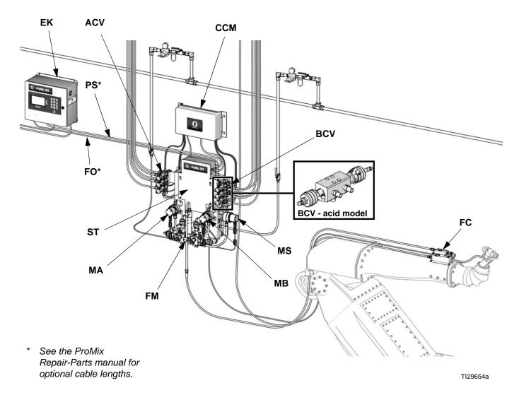
Fig. 3. Wall Mount System, shown with G3000 Meters, Color/Catalyst Change, Accessory Solvent Meter, and Flow Control
