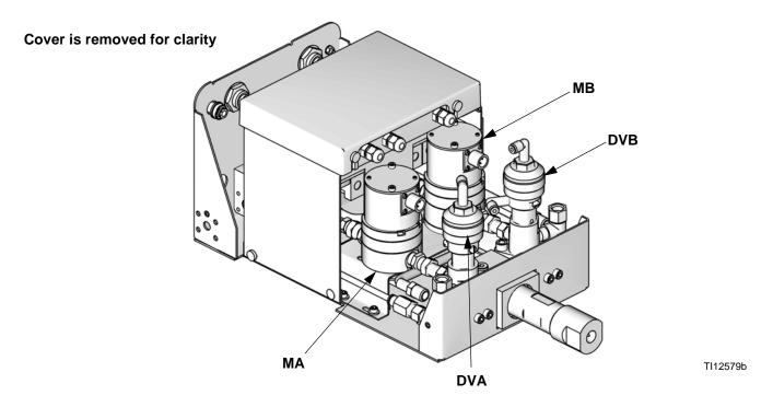
Fig. 6: Details of RoboMix Fluid Station
