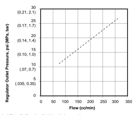
Fig. 99. Typical Flow Calibration (0-300 cc/min range)
