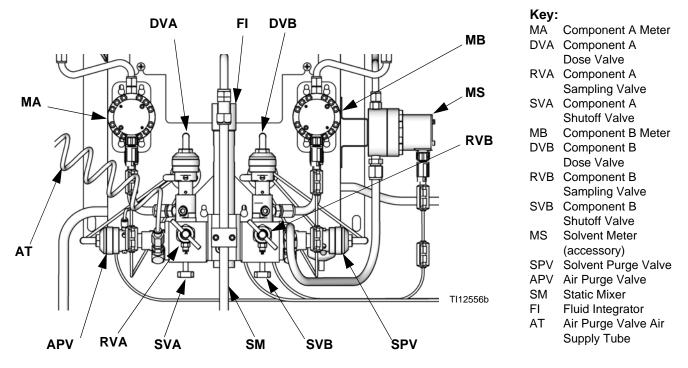
Fig. 119. Wall Mount Fluid Station
