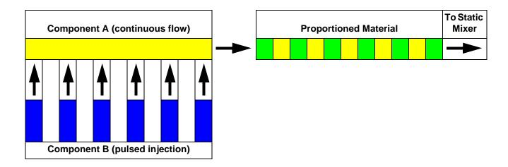
Fig. 105. Schematic Diagram of Dynamic Dosing Operation
