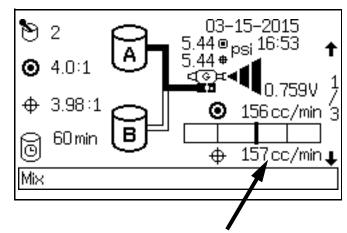
Fig. 115. Status Screen Flow Rate Display
