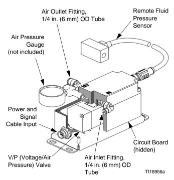
Fig. 85. Cutaway of 24H989 Flow Control Module
