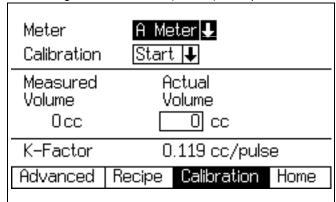
Fig. 120. Calibration Screen
