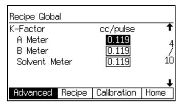
Fig. 43. Advanced Setup Screen 4
