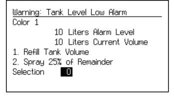
Fig. 22. Tank Level Low Screen (Tank A Shown)
