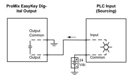
Fig. 76. Automation 24 Vdc Sourcing Input Diagram
