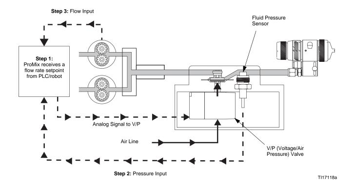
Fig. 88. ProMix Flow Control Pressure Loop and Flow Loop (249849 Module)
