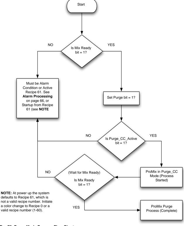
Fig. 73. Purge Mode Process Flow Chart
