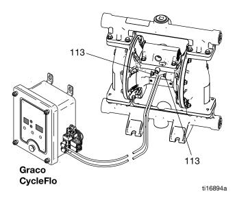
FIG. 2. Connect Remote Air Control
