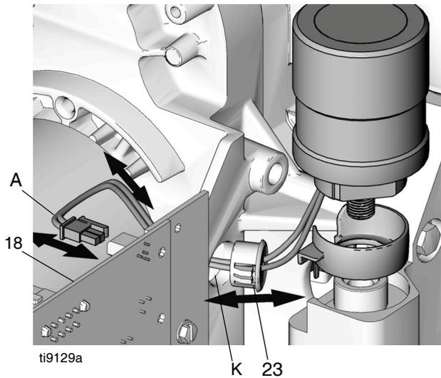
7. Pull wires through hole (K).
