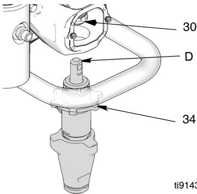
2. Install pump rod (D) into connecting rod (30).
