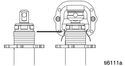
6. Align pump outlet (E) to back.
