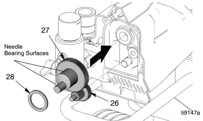
2. Push drive housing (29) into motor front endbell. Insert gear crank (27) through hole in connecting rod (30).
