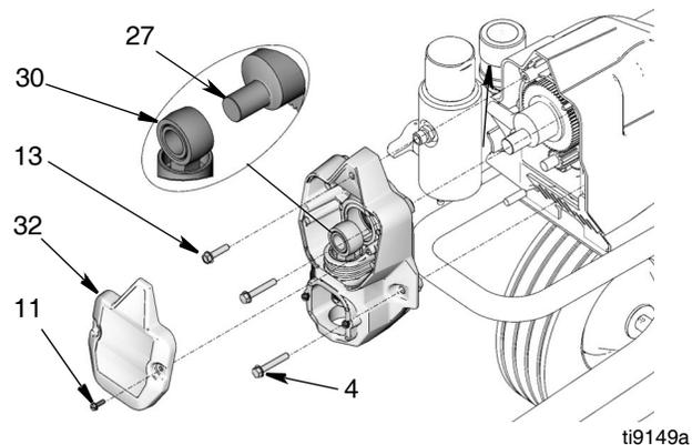
3. Install four screws (4) and screw (13).
