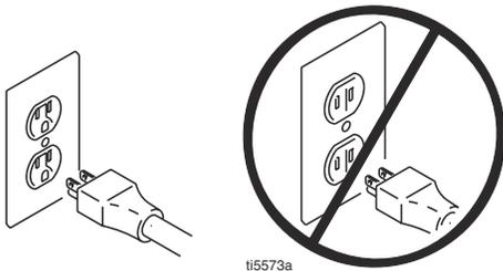
Do not use the sprayer if the electrical cord has a damaged ground contact. Only use an extension cord with an undamaged ground contact.
