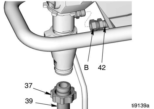
9. Fill packing nut with Graco TSL until fluid flows onto top of seal. Install pail hanger (10) with screws (11).
