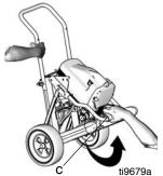
Install hose rack (d) to frame handle. Install lock nuts. Tighten securely.
