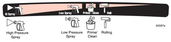
**NOTE:** To select function, align symbol on pressure control knob with setting indicator on sprayer.
