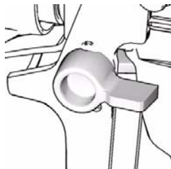
Trigger Locked (no spray)
