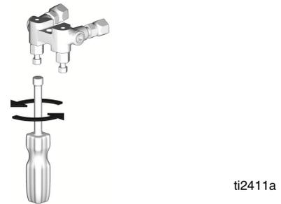
**10. Connect whip hose to gun fluid manifold**
