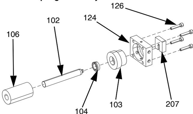
7. Lubricate the dispense sleeve bore in the valve body (107). Insert the rod sleeve (106) into the main body (107).
