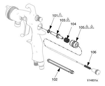
U-cup (101) must be installed with supplied tool. Apply pressure until it clicks into place.
