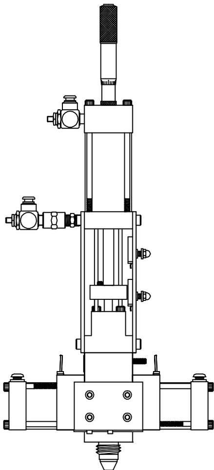
**FIG. 2: PD44 Micrometer Dispense Valve**
