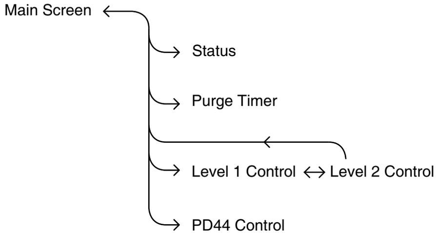
FIG. 6: Screen Navigation Diagram
