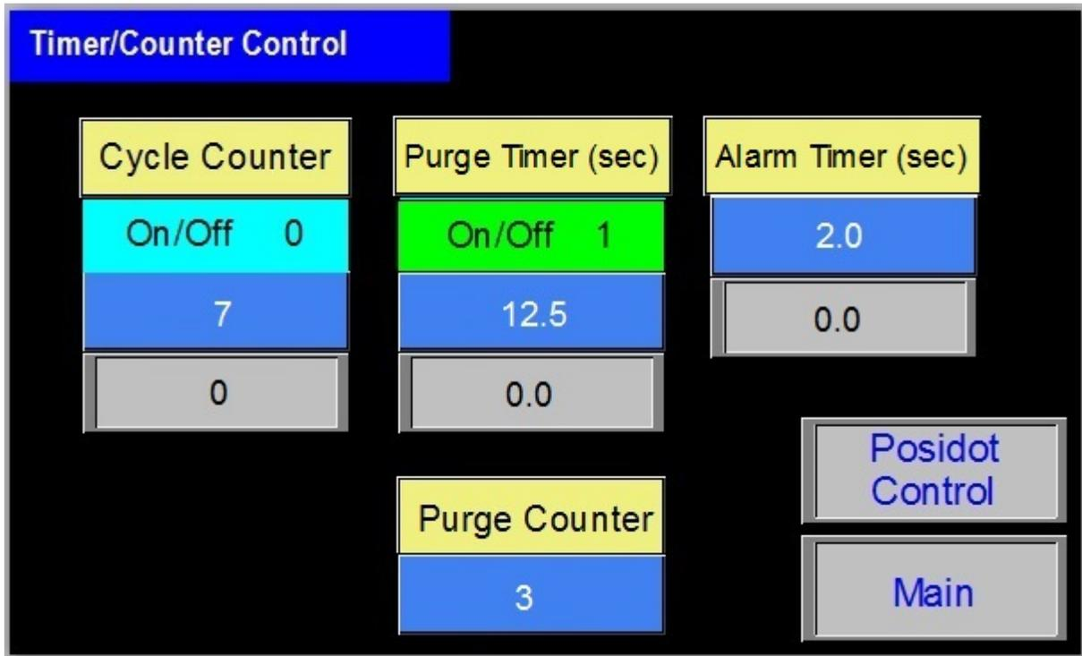
FIG. 9: Timer/Counter Control Screen
