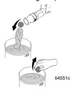
10. Turn on/off switch OFF and turn prime/drain valve to DRAIN. Clean outside of pump and suction tube with brush and water.
