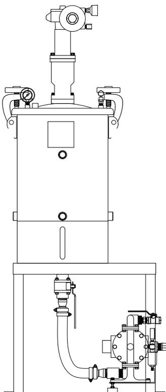
10 Gallon Tank with Diaphragm Pump, Agitator,
