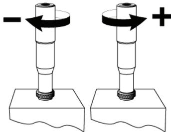
3. Rotate the shot size locking ring clockwise to tighten.
