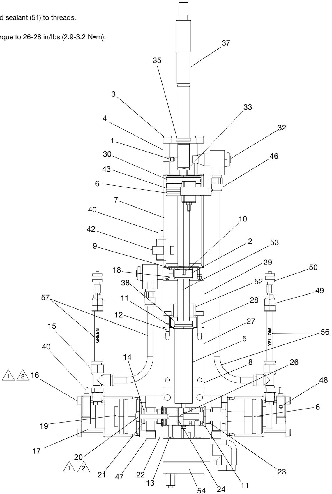
**1092 Valve Components, 3" Stroke CD**
