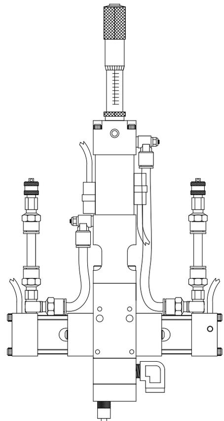
*Cycle Detection and Luer Lock Outlet Shown*
