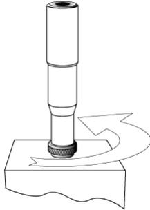
2. Rotate the shot size adjuster to adjust shot size.
