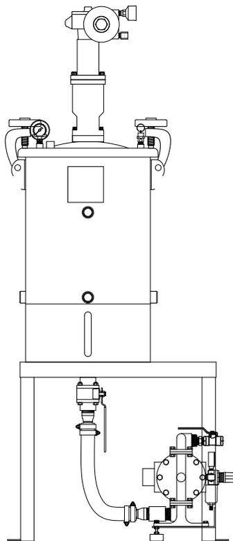
*10 Gallon Tank with Diaphragm Pump, Agitator,
