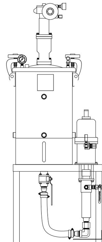
*10 Gallon Tank with 5:1 Pump, Agitator, Vacuum,
