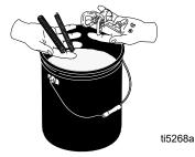
5. Remove siphon tube set from paint and place in flushing fluid. Use water for water base paint and mineral spirits for oil base paint.
