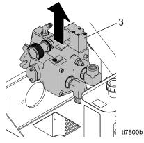
12. Remove fittings (30, 34, 35) from pump (3) and set aside to use on the new pump.
