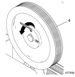
9. Remove pulley (4) from hydraulic pump shaft.
