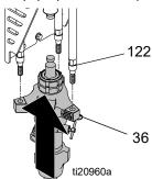
Screw tie rod locknuts (213) onto tie rods. Torque to 50 +/- 8 ft-lb (68 +/- 11 N•m)
