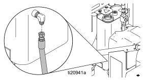
5. Reattach return lines (100, 101). Torque three times to 450 <u>+</u> 10 in-lb (51 <u>+</u> 1.1 N•m).
