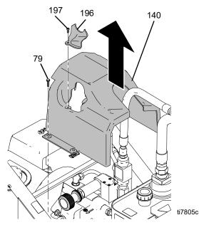
3. Remove compensator screws and separate compensator and adapter block.
