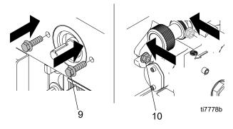
4. Replace large pulley (4) on hydraulic pump shaft.
