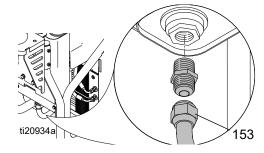
8. Verify drain plug has been replaced. Fill oil reservoir with oil to high mark on dip stick (approximately 3.5 gallons).
