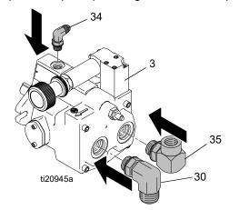
**NOTE**: Fill pump casing with hydraulic oil before installing fitting (34).
