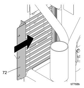
2. Replace bar and screws. Torque to 25-30 in-lb (2.8-3.4 N•m).
