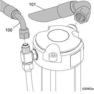
7. Remove cooler line from reservoir (64).
