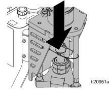
Tighten power head bolts (7). Torque bolts to 400 <u>+</u> 10 in-lb (45 <u>+</u> 1 N•m).
