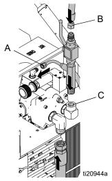
Install cover (140) and with four screws (79). Torque to 25-30 in-lb (2.8 - 3.4 N•m). Install pump handle cover (196) with screw (197).
