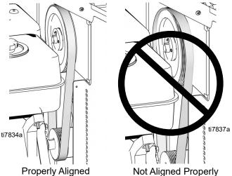
OTE: If belt is not aligned properly, to adjust
