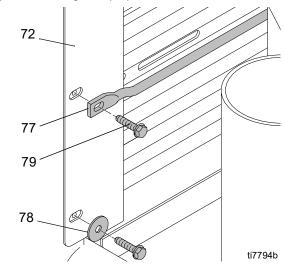
5. Remove coil (72) from sprayer frame.
