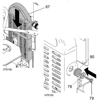
Install suction lines. Tighten fittings. Torque fitting A to 225 <u>+</u> 10 in-lb (25.4 <u>+</u> 1.1 N•m). Fitting B to 450 <u>+</u>10 in-lb (50.1 <u>+</u> 1.1. N•m). Fitting C to 225 in-lb (25.4 N•m).
