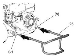
6. Install sleeve screws (143) in lower frame tubes.
