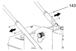
2. Remove handle assembly (25) by pulling it out of upper frame tubes (1).
