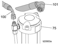
4. To purge air from hydraulic lines, increase pressure enough to start hydraulic motor stroking and allow fluid to circulate for 15 seconds.Turn pressure down. Close prime valve.
