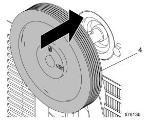
5. Align pulley (4) on shaft. When properly positioned approximately 1/8 inch of shaft (139) will protrude.
