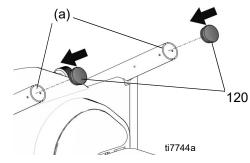
Insert handle assembly (25) into lower frame tubes (b). The hose bracket should face down. Adjust to appropriate in/out location.
