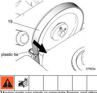
Moving parts can pinch or amputate fingers and other body parts. To avoid serious injury be sure engine is in OFF position before pulling engine recoil.
