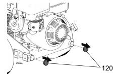
4. Insert plugs (120) in upper frame handle tubes (a).
