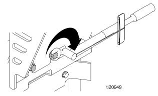
Attach hoses (100, 101) to head (75). Torque to 450 <u>+</u> 10 in-lb (50.84 N•m).
