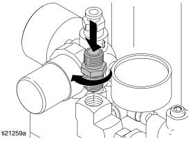
10. Use wrench to install second regulator assembly (G) and position as shown below.
