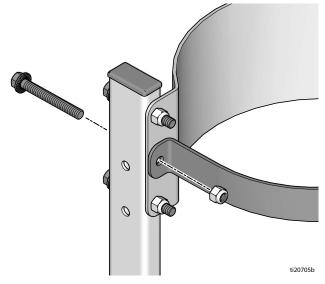
4. Remove 1.25 in. bolt (C) from center strap mounting hole. **NOTE:** The bolt will be used to secure both straps once the second bead tank is in place.
