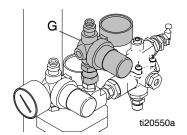
Install 36 in. nylon air line from top of second regulator (G) to swivel fitting on top of second bead tank. Push airline into each fitting as shown.
