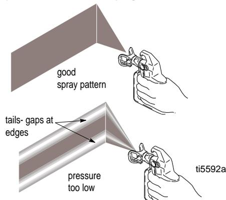
**NOTE:** If tails persist when spraying at the highest pressure, a smaller tip is needed or the material may need to be thinned.
