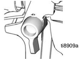
5. When obstruction is cleared, engage trigger lock and rotate arrow-shaped handle back to SPRAY position.
