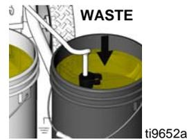
8. Submerge suction tube in water
