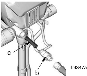
4. Tighten outlet fitting and reconnect hose (a) to sprayer. Use two wrenches to tighten securely.
