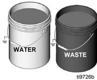
4. Lift suction tube and prime tube from paint pail. Let them drain into paint pail for a while.
