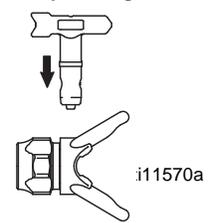
3. Screw tip and guard assembly on gun. Tighten retaining nut.
