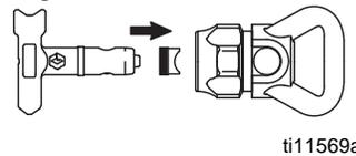
Tip must be pushed all the way into guard
