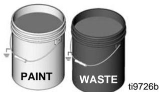
4. Lift suction tube and prime tube from paint pail. Let them drain into paint for a while.
