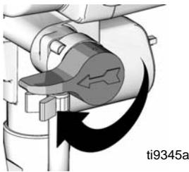
**NOTE:** Some fluids may prime faster if the Power Switch is momentarily turned off so the pump can slow and stop. Repeat several times if necessary.
