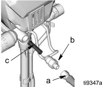
3. Check InstaClean™ Fluid Filter (c) for debris. If needed, clean filter with water and a soft brush.
