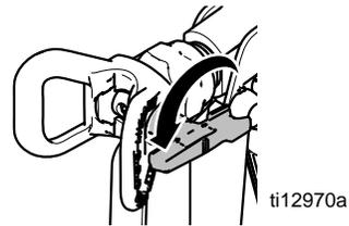
HINT: Point the arrow-shaped handle on the spray tip forward to SPRAY and backward to UNCLOG obstructions.
