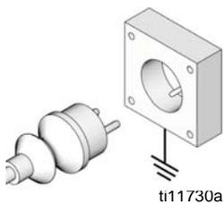
**Spray gun:** ground through connection to a properly grounded fluid hose and pump.
