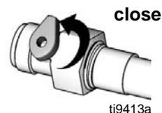
22. Unscrew Power Flush attachment from suction tube.
