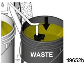
7. Submerge suction tube in water
