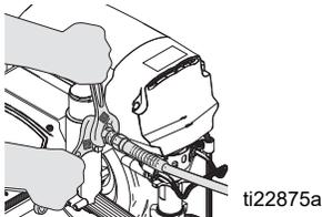
If using the optional hopper, remove the nipple fitting from the filter. Install 45° elbow (from parts box) into filter and install nipple fitting into elbow. Then connect the hose to the nipple.
