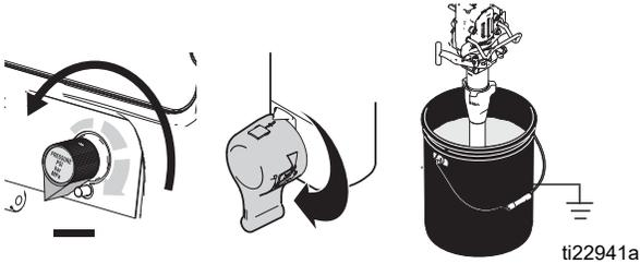
2. Turn power ON. Pressure display appears. Dashes will not appear unless pressure is less than 200 psi (14 bar, 1.4 MPa).
