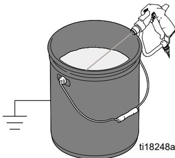
5. Turn prime valve down to **DRAIN** position and allow flushing fluid to circulate until flushing fluid appears clear.
