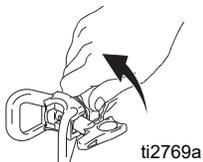
5. Check inlet strainer for clogs and debris.
