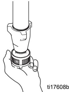
6. Fill throat packing nut with Graco TSL to prevent premature packing wear. Do this each time you spray.
