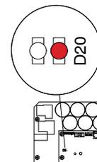
For units without a display, see **ProGuard** (page 18). If there is a voltage supply issue (CODE 04, 08, or 17), the ProGuard status light will blink continuously when the ON/OFF switch is ON. To determine which code (or any other code besides voltage supply) refer to the control board status light. Turn the ON/OFF switch OFF, remove the control cover then turn power back ON. Observe the status light. Blinking LED total count equals the error code (for example: two blinks equals CODE 02).
