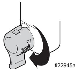
9. Remove filters from gun and sprayer, if installed. Clean and inspect. Install filters.
