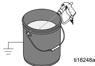
10. Engage trigger lock. Assemble tip and guard, see instructions on next page.
