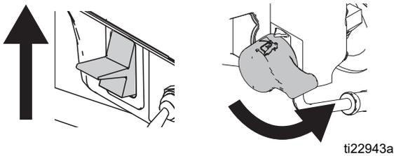
3. Increase pressure to 1/2. Hold gun against pail. Disengage trigger lock. Trigger gun until flushing fluid appears.
