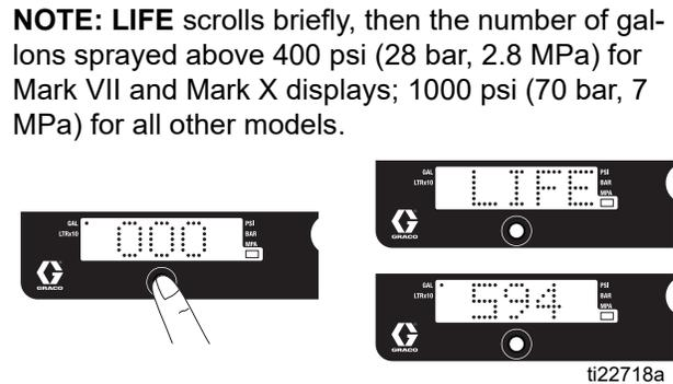
**NOTE:** **LIFE** scrolls briefly, then the number of gallons sprayed above 400 psi (28 bar, 2.8 MPa) for Mark VII and Mark X displays; 1000 psi (70 bar, 7 MPa) for all other models.
