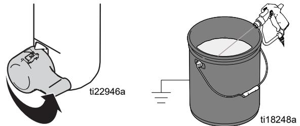
7. Raise pump above flushing fluid and run sprayer for 15 to 30 seconds to drain fluid. Turn power **OFF**.
