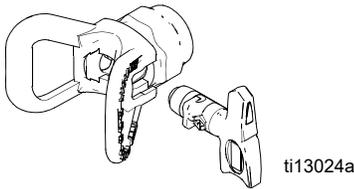
4. Screw assembly onto gun. Tighten.
