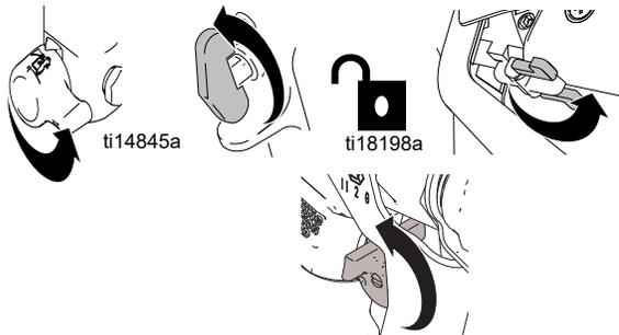
6. Hold gun against grounded metal flushing pail. Trigger gun and increase fluid pressure 1/2 turn. Flush 1 minute.
