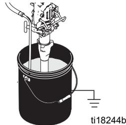
9. Trigger gun again into flushing pail until paint appears. Move gun to paint pail and trigger for 20 seconds.
