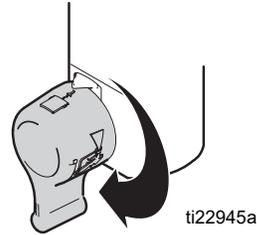
6. Turn prime valve forward to **SPRAY** position. Trigger gun into flushing pail to purge fluid from hose.
