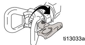
2. Engage trigger lock. Return SwitchTip to original position. Disengage trigger lock and continue spraying.
