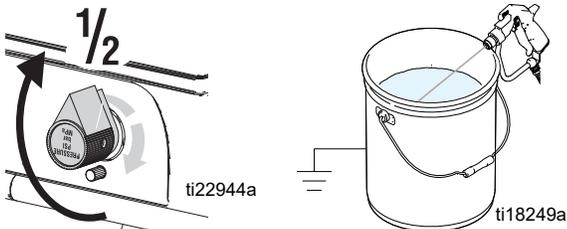
4. Move gun to waste pail, hold gun against pail, trigger gun to thoroughly flush system. Release trigger and engage trigger lock.
