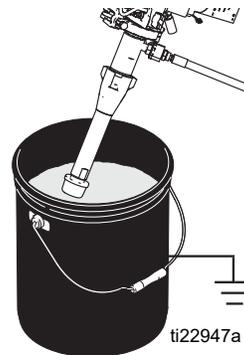
8. Turn prime valve down **DRAIN** position. Unplug sprayer.
