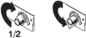
5. Turn prime valve forward to **SPRAY** position. Disengage trigger lock.
