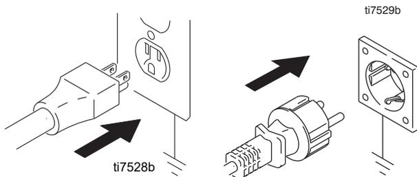
Do not modify plug! If it will not fit in outlet, have grounded outlet installed by a qualified electrician. Do not use an adapter.
