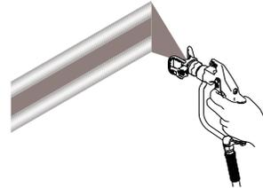
2. Hold gun perpendicular, 10-12 in. (25-30 cm) from surface. Spray back and forth. Overlap by 50%. Trigger gun after moving and release before stopping.
