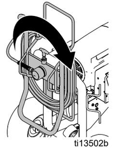
**NOTE:** The hose reel can be locked into two positions: Usage (A) and Storage (B).
