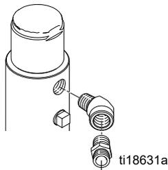
**NOTE:** Make sure nipple fitting is angled away from hopper so the hose can be easily installed.
