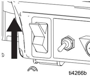
4. Increase pressure 1/2 turn to start motor and allow fluid to circulate through drain tube for 15 seconds; turn pressure down.
