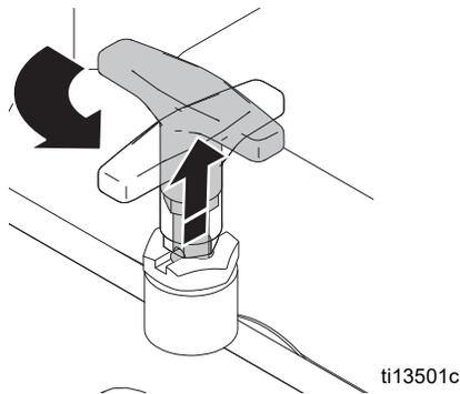
3. Pull reel handle up and turn clockwise to reel in hose.
