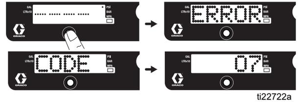
8. Press and hold DTS button to clear code to zero.
