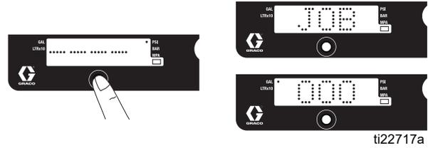
**NOTE:** **JOB** scrolls past, then the number of gallons sprayed above 400 psi (28 bar, 2.8 MPa) for Mark VII and Mark X displays; 1000 psi (70 bar, 7 MPa) for all other models.
