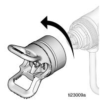
2. Install spray tip into cap assembly.
