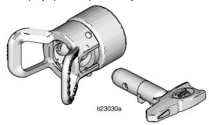
3. Remove diffuser assembly with gun tool.
