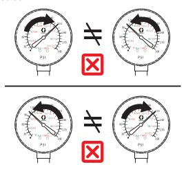
The most typical time for pressure variations to occur is right after the top change over. This pressure variation is caused by one of the double acting piston pumps "A" or "B" cavitating during the up, or fill stroke, and then not having fluid to pump until it travels down to the filled level. Cavitation causes ratio errors and should not be allowed at any time while spraying.
