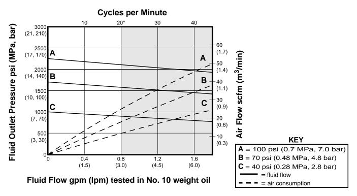
7.5" Air Motor with 4:1 Lower Pump Ratio 125 cc/cycle
