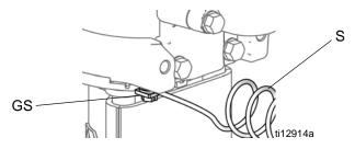
Fig. 4. Ground screw and wire
