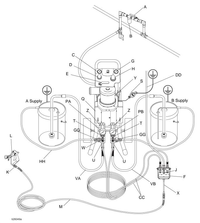
Fig. 3 Typical Installation, Polyester Model
