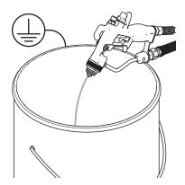
16. Engage trigger lock. Install the spray tip and/or air cap. Disengage trigger lock and trigger gun to flush tip and/or air cap with solvent. Engage trigger lock and remove the spray tip and/or air cap.
