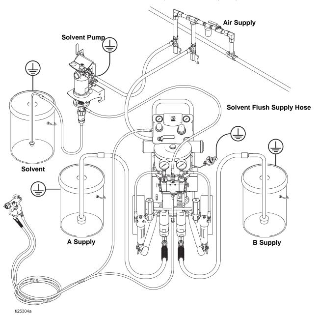
Fig. 1 Typical System Installation
