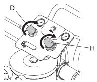
11. Disengage the gun trigger lock and spray. See **Spray Gun Adjustment**. page 22.
