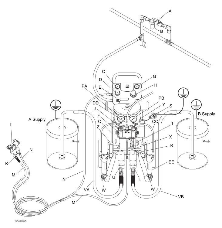
Fig. 2 Typical Installation, Non-Polyester Models
