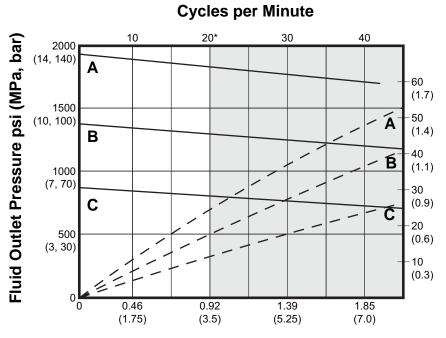
Fluid Flow gpm (lpm) tested in No. 10 weight oil
