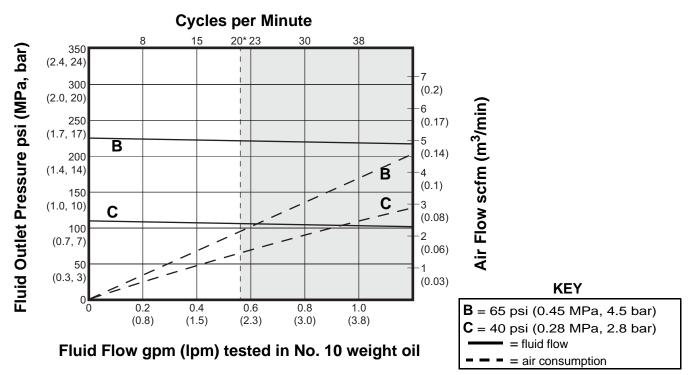
2.5" Air Motor with 2:1 and 5:1 Lower Pump Ratio 150 cc/cycle
