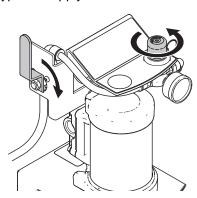
Disengage the trigger lock and trigger the gun into a grounded metal waste pail until flow stops and pressure is relieved.
