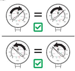
If one pressure or the other increases while the other decreases the proportioner is not working correctly. The cause should be determined and corrected.
