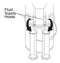
Fig. 5 Checking Mix Ratio
