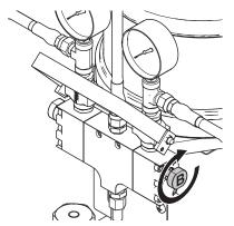
18. Turn off air regulator to solvent pump. Close the bleed type air supply valve to the solvent pump.
