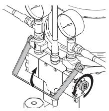
7. Open bleed type air valve on the solvent pump to provide air to flush the pump. Increase air pressure regulator on solvent pump.
