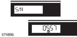
5. Press and hold DTS button to clear error code to zero. Short press to move to software **REV**.
