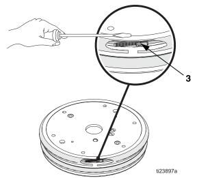
5. Work hose to completely close gap at the ends.
