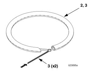
NOTE: To prevent material from potentially leaking past both hoses, ensure hose (1,2) seams are 90°-180° apart, and not on top of each other.
