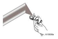
Hold gun perpendicular, 10-12 in. (25-30 cm) from surface. Spray back and forth. Overlap by 50%. Trigger gun after moving and release before stopping.
