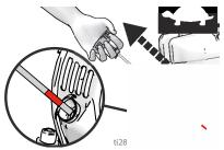
Without releasing the starter rope C. handle allow the rope to rewind completely.
