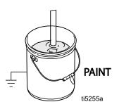
13. Trigger gun again into flushing fluid pail until paint appears.
