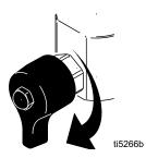
Raise siphon tube above flushing fluid and run sprayer for 15 to 30 seconds to drain fluid. Turn hydraulic valve OFF. Turn engine OFF or turn electric motor OFF and unplug.
