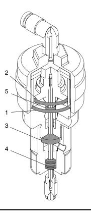
**NOTE:** Lubricate all o-rings, seals and internal bores prior to installation.
