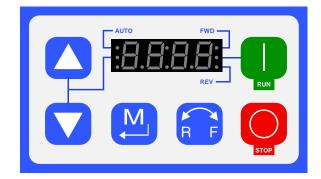
Figure 15 VFD Control Panel
