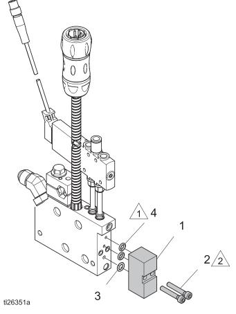
Apply high temperature lubricant (6) to o-rings (3 and 4).
