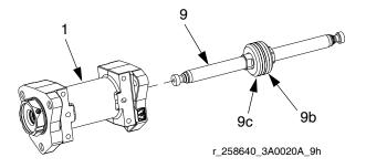
9. Install second seal housing (2) on cylinder (1). Torque to 150-160 ft-lbs (203-216 N•m).
