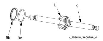
3. Install sealing ring of bidirectional seal (9b) over rub ber energizing ring and install bearing (9c) in shal low piston groove.
