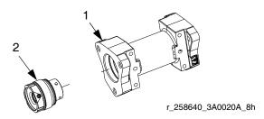
Install piston rod assembly (9) in cylinder (1) with bidirectional seal (9b) facing away from the cylinder (1). Apply hydraulic oil to bidirectional seal and bearing (9c). Use rubber mallet to tap piston rod assembly until the piston is approximately at the middle of the cylinder.
