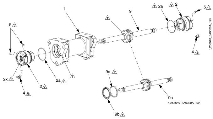
1 Lubricate seals and surfaces with hydraulic oil.
