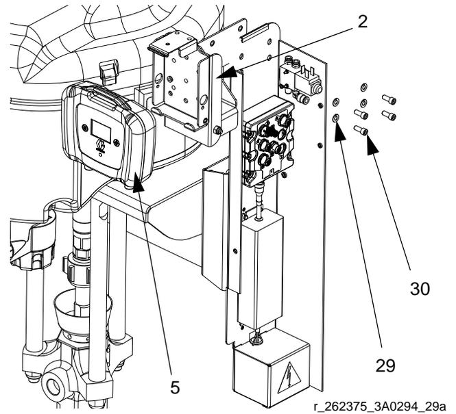
**FIG. 83: Install Display Bracket**
