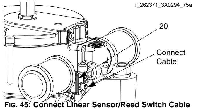
**FIG. 45: Connect Linear Sensor/Reed Switch Cable**
