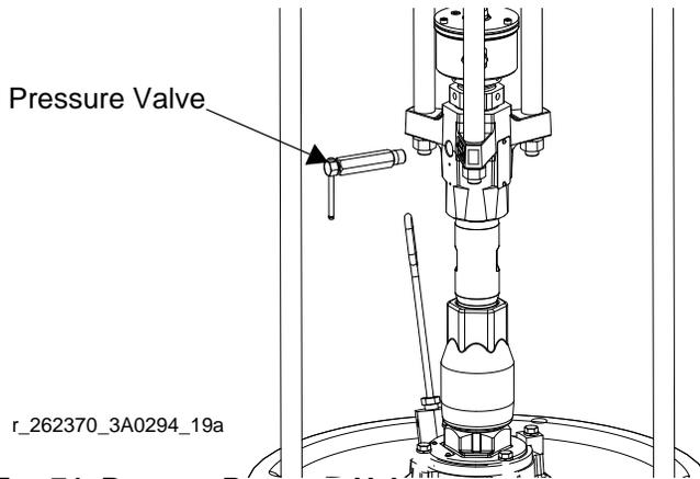
**FIG. 74: Remove Pressure Valve**
