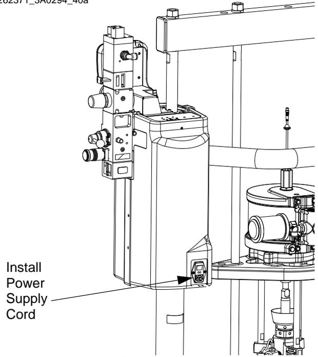
**FIG. 48: Install Power Supply Cord**
