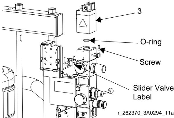
**FIG. 16: Install Air Valve Assembly**
