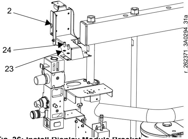
**FIG. 36: Install Display Module Bracket**
