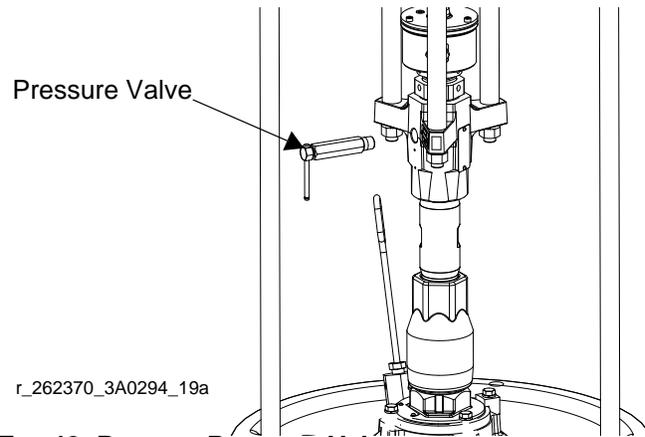
**FIG. 42: Remove Pressure Valve**
