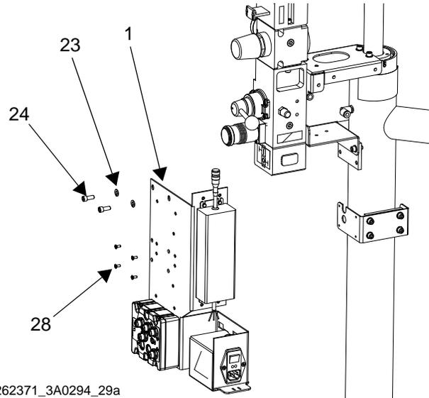
**FIG. 34: Install Electronics Assembly**
