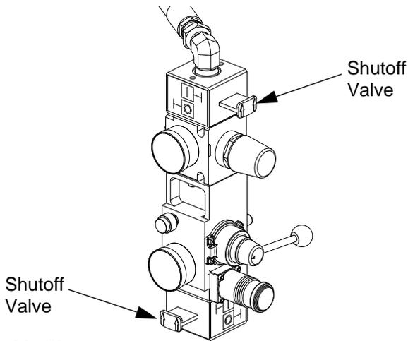
**FIG. 32: Close Shutoff Valves**
