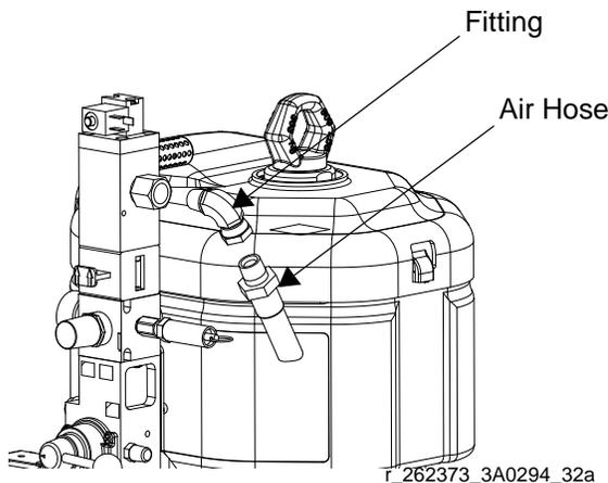
**FIG. 54: Install Fitting and Air Hose**
