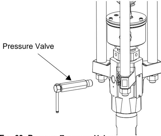
**FIG. 60: Remove Pressure Valve**
