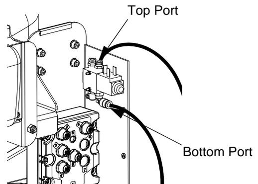
**FIG. 97: Install Air Lines - Solenoid Valve**
