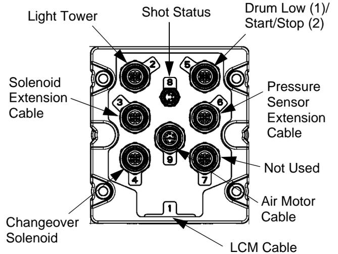
**FIG. 62: Breakout Module Connections**
