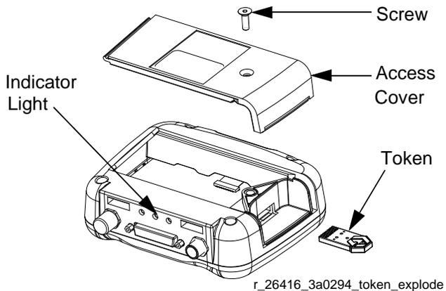
**FIG. 105: Upgrade Display Software**
