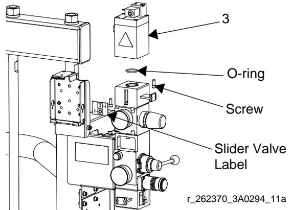
**FIG. 38: Install Air Valve Assembly**
