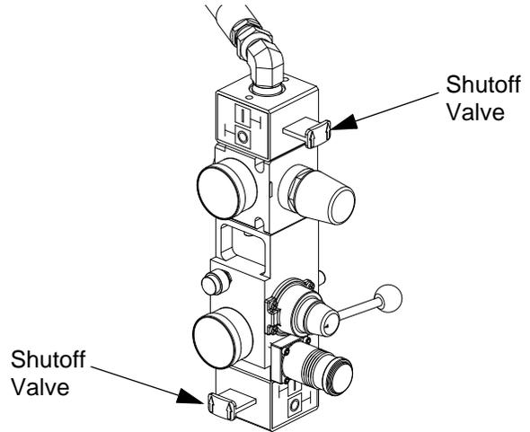
**FIG. 10: Close Shutoff Valves**
