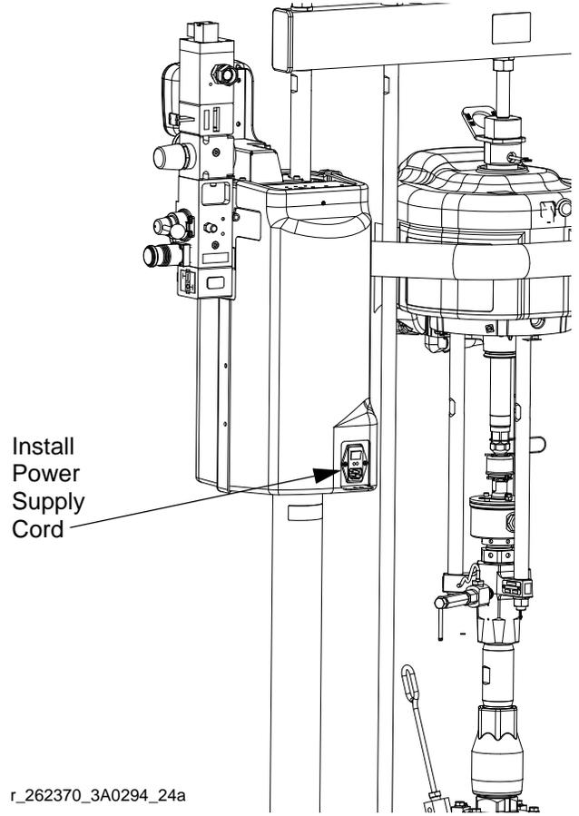
**FIG. 31: Install Power Supply Cord**
