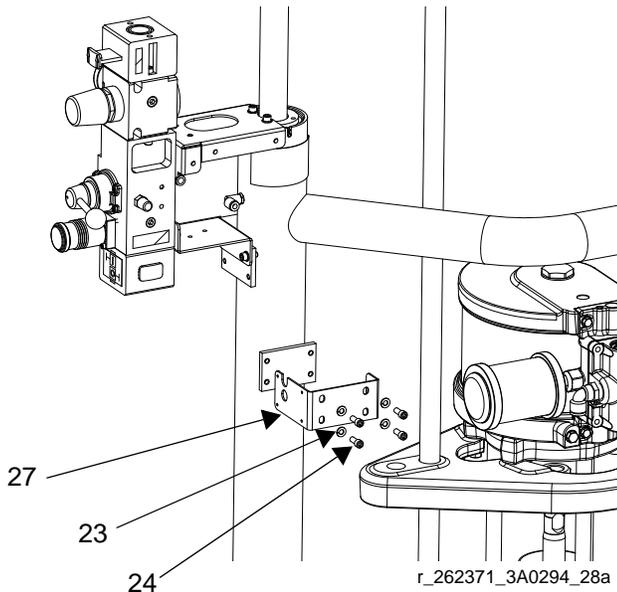
**FIG. 33: Install Power Supply Bracket**
