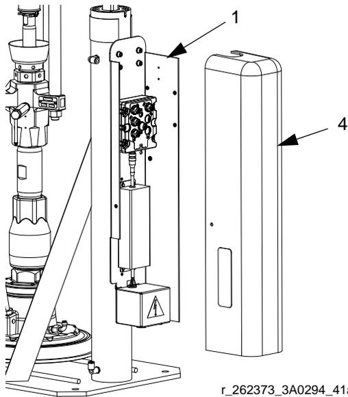
**Fig. 64: Install Electronics Cover**
