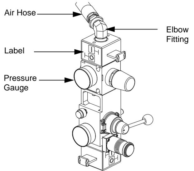
**FIG. 15: Air Control Assembly**
