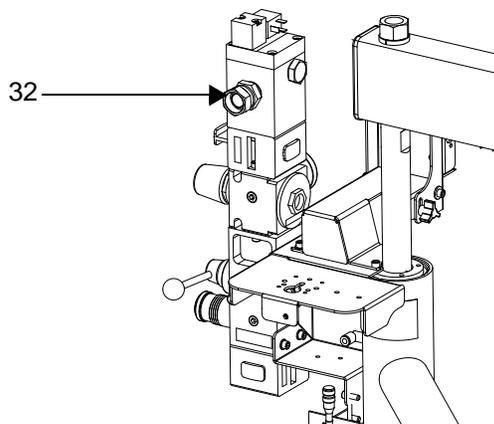
**FIG. 17: Install Swivel Fitting**
