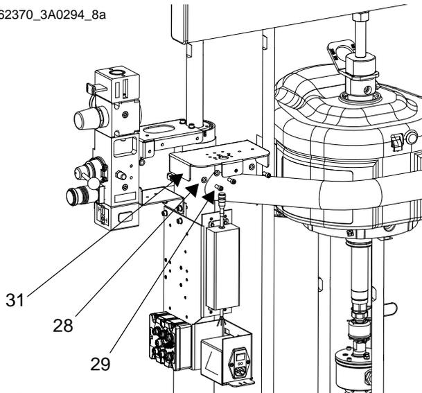
**FIG. 13: Install Light Tower Bracket**
