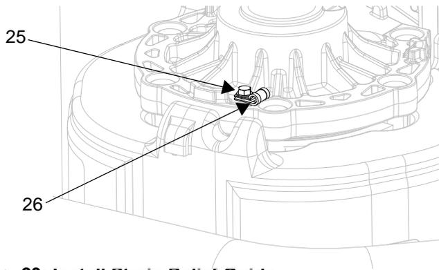
**FIG. 23: Install Strain Relief Guide**
