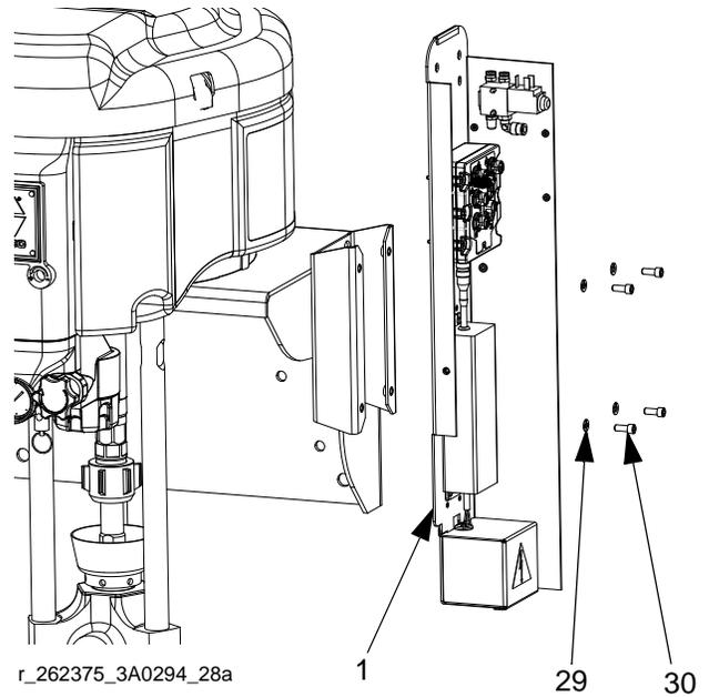
**FIG. 82: Install Electronics Assembly**
