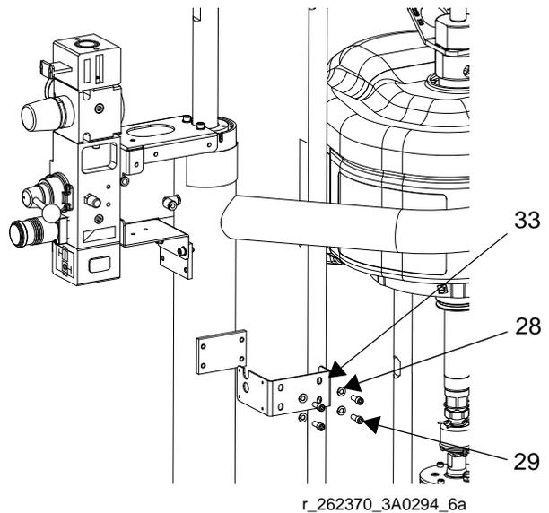
**FIG. 11: Install Power Supply Bracket**
