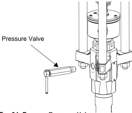
**FIG. 94: Remove Pressure Valve**
