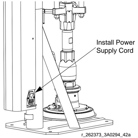
**Fig. 65: Install Power Supply Cord**
