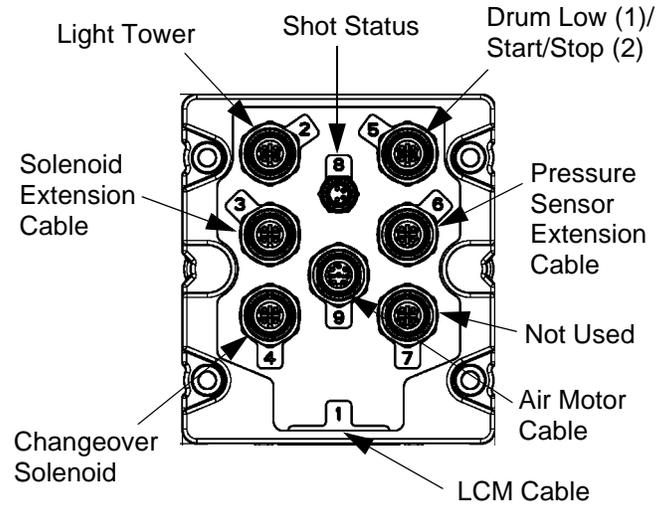
**FIG. 28: Breakout Module Connections**
