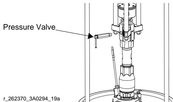
**FIG. 26: Remove Pressure Valve**
