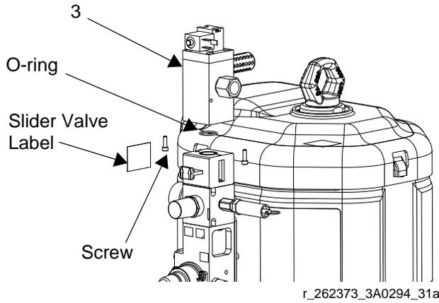
**FIG. 53: Install Air Valve Assembly**
