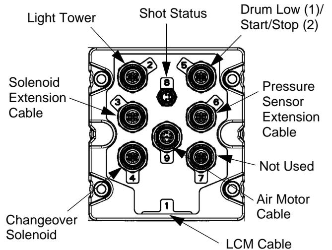
**FIG. 76: Breakout Module Connections**
