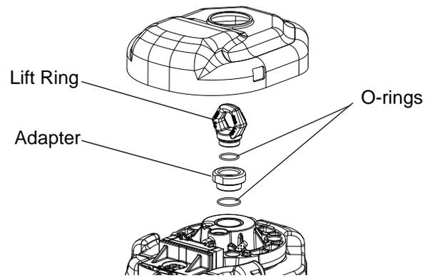
**FIG. 56: Remove Lift Ring Adapter and O-rings**
