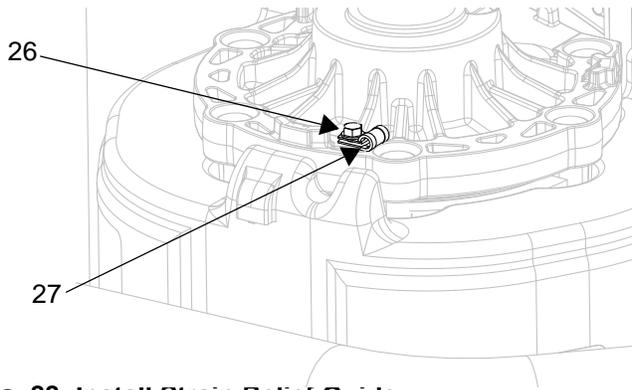
**FIG. 88: Install Strain Relief Guide**
