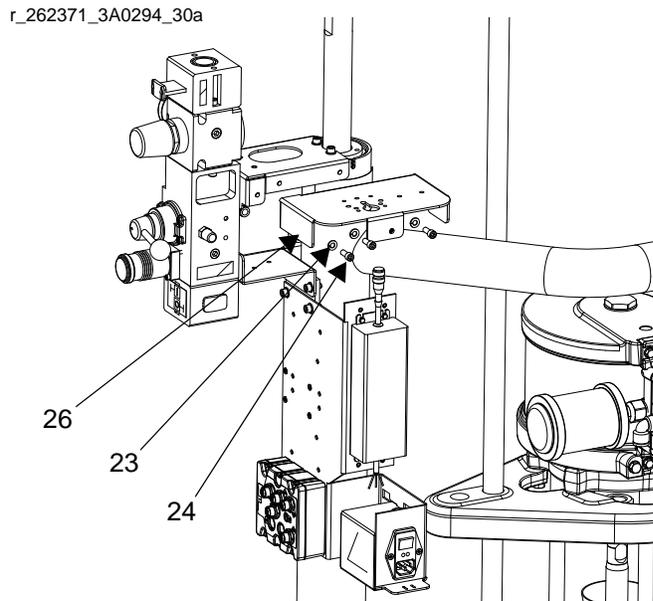
**FIG. 35: Install Light Tower Bracket**
