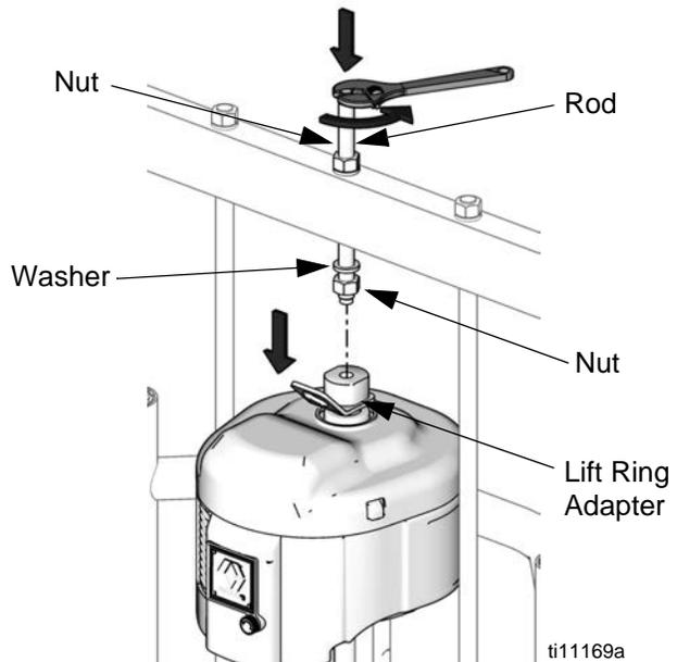
**FIG. 25: Reconnect Air Motor**
