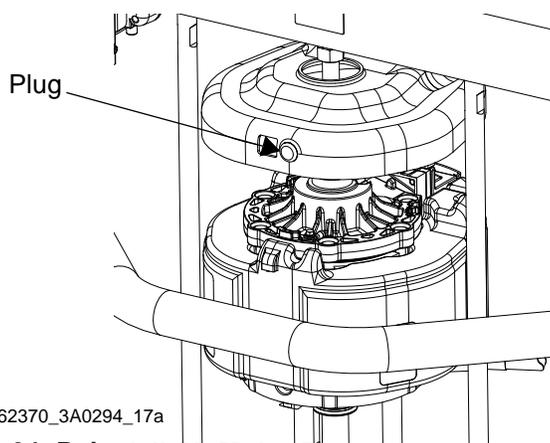
**FIG. 24: Reinstall Air Motor Cover**
