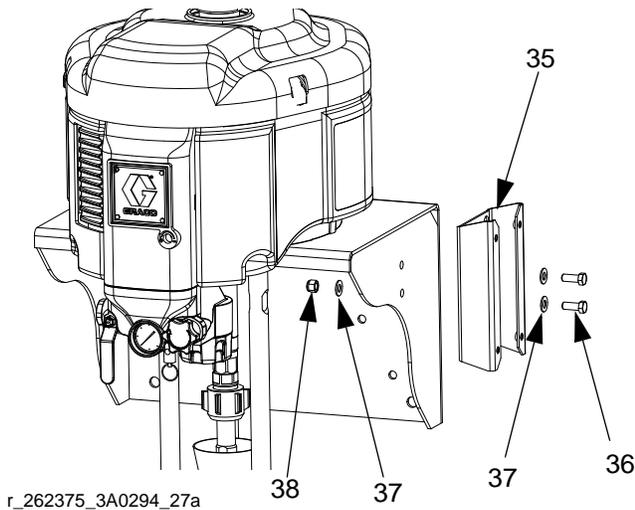
**FIG. 81: Install Adapter Bracket**
