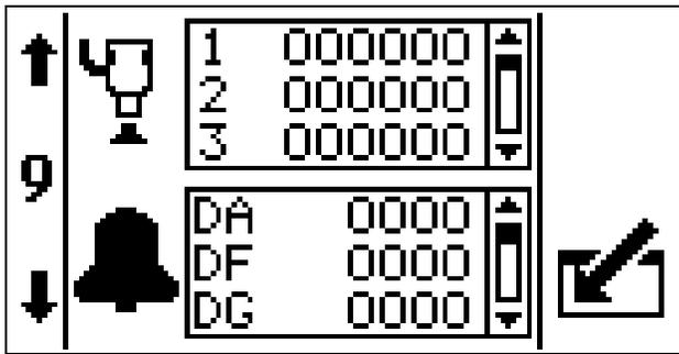
Shot and error totalizer screen shown with shot number highlighted, which enables the user to clear a shot by then pressing  $\begin{matrix} 123 \\ \downarrow \\ 000 \end{matrix}$ .
