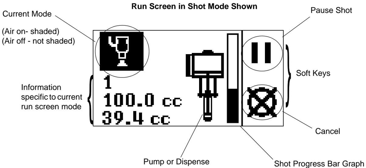
**FIG. 7: Run Mode Screen Components**
