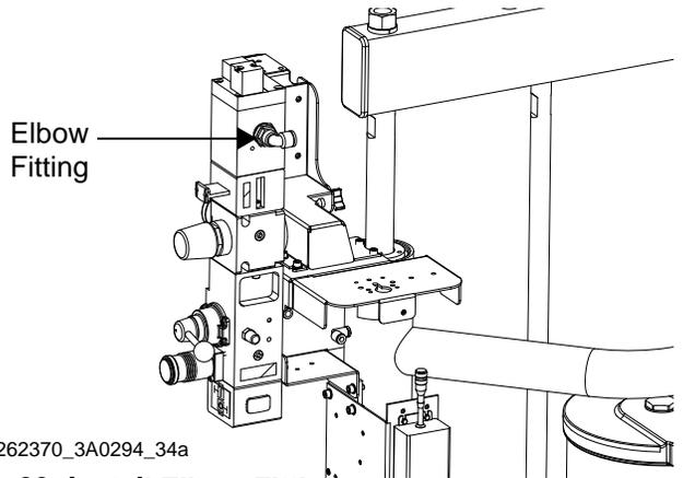
**FIG. 39: Install Elbow Fitting**
