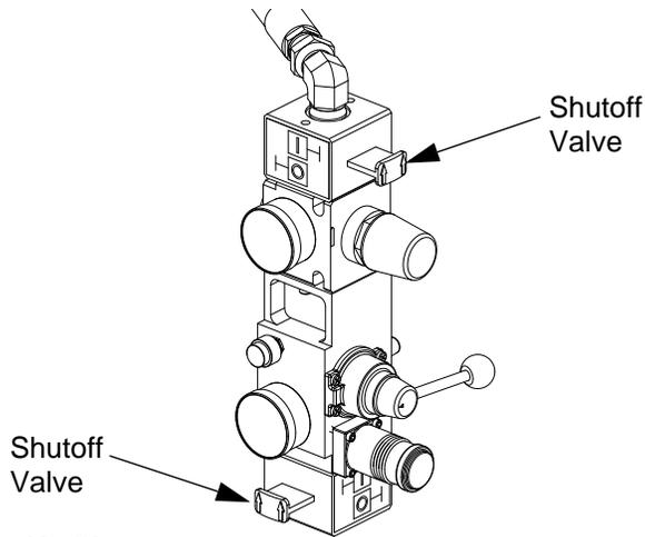
**FIG. 49: Close Shutoff Valves**
