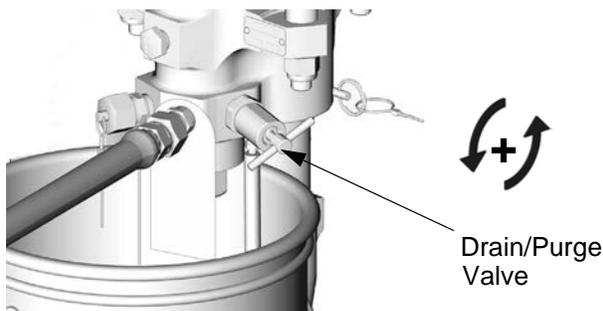
**FIG. 102: Drain Material**
