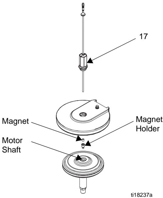
**FIG. 40: Install Linear Sensor**
