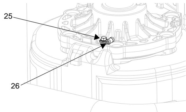
**FIG. 59: Install Strain Relief Guide**
