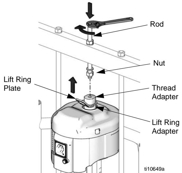
**FIG. 18: Disconnect Air Motor**
