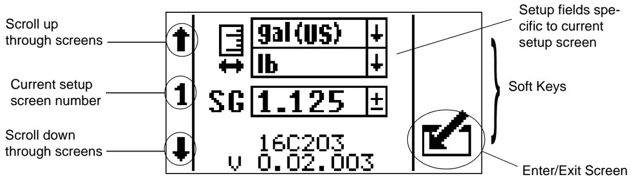
**FIG. 6: Setup Mode Screen Components**
