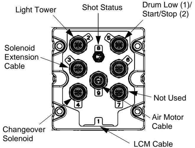
**FIG. 92: Breakout Module Connections**
