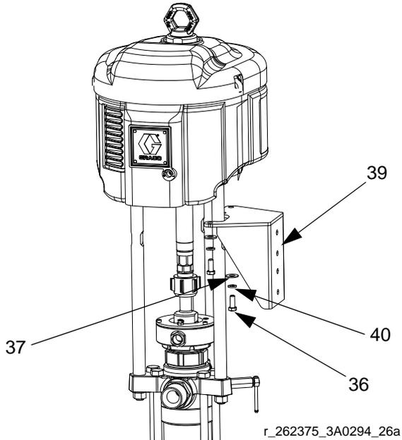
**FIG. 80: Install Control Mount Bracket**
