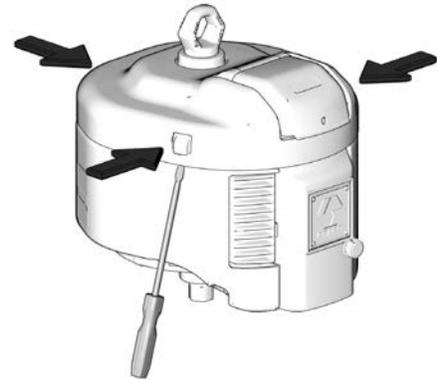
**FIG. 55: Remove Air Motor Cover**
