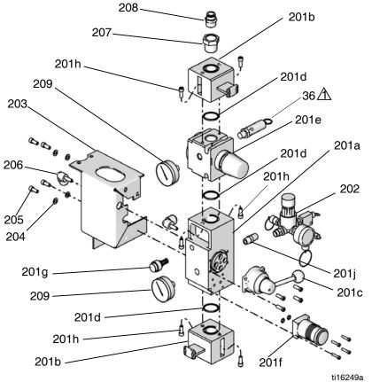
$\bigtriangleup$  The safety valve is part of the ram package. See page 21 (piston pump packages).
