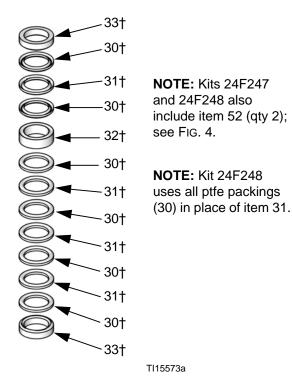
Fig. 5. Throat Packing Detail (3000cc and 4000cc)
