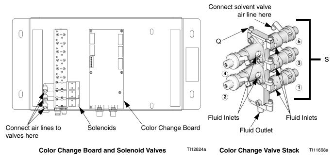
Fig. 7. Color Change Valves Air and Fluid Connections
