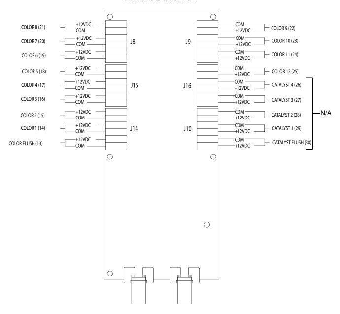
Fig. 13. Color Change Module Electrical Schematic
