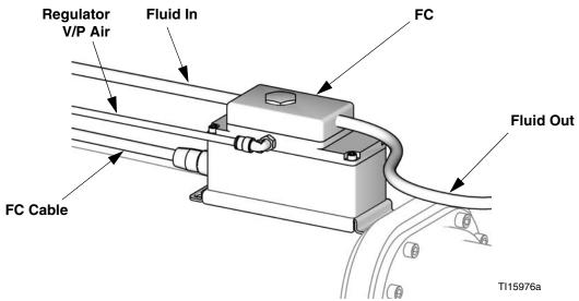
Fig. 8. Flow Control Regulator
