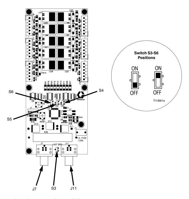
Fig. 12. Color Change Board Switches S3-S6
