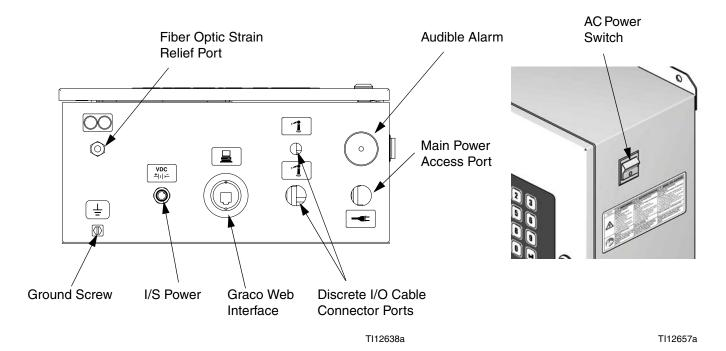
Fig. 10. EasyKey Connections and AC Power Switch
