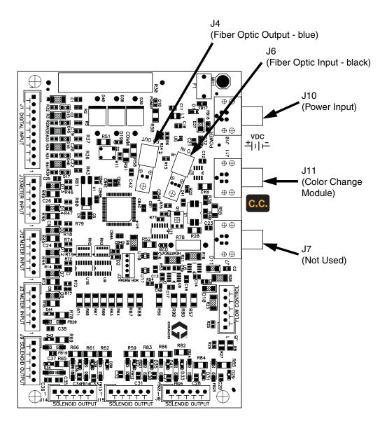
Fig. 11. Fluid Station Board Connections
