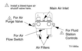
Fig. 5. Air Supply Control
