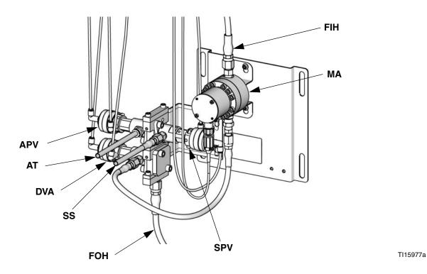
Fig. 6. Fluid Manifold
