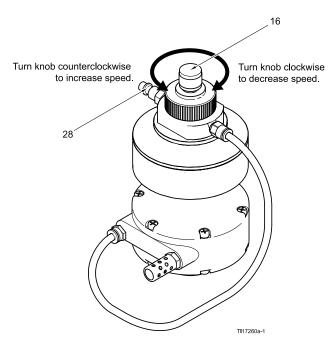
To shut off the agitator, disconnect the air supply or turn the speed adjustment knob clockwise until it is fully closed.
