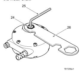
5. Ensure that the drive shaft hex (C) engages the hex socket (D) in the flange connector. Screw the base of the speed controller into the threads at the top of the air motor until hand tight.
