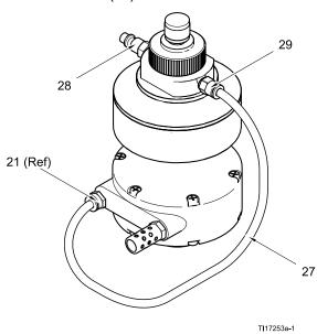
7. Return the unit to service. Connect the main air line to the quick-disconnect fitting (28) on the speed controller.
