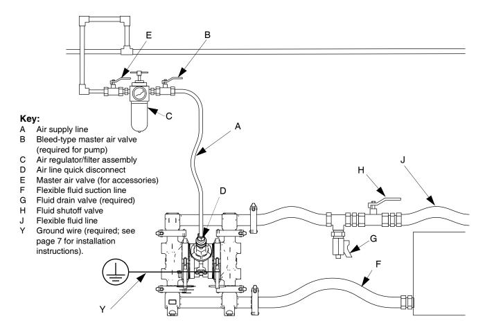
Fig. 2: Typical Floor-Mount Installation
