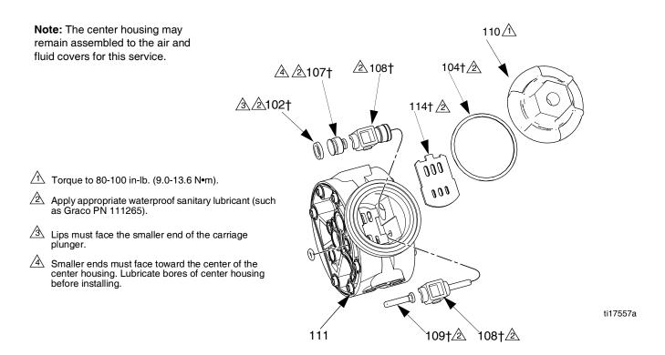
Fig. 5. Disassemble/Reassemble the Air Valve
