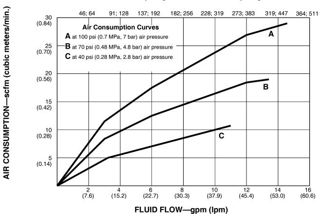
**To find Pump Air Consumption** (scfm or m<sup>3</sup>/min) at a specific fluid flow (gmp/lpm) and operating air pressure (psi/MPa/bar):
