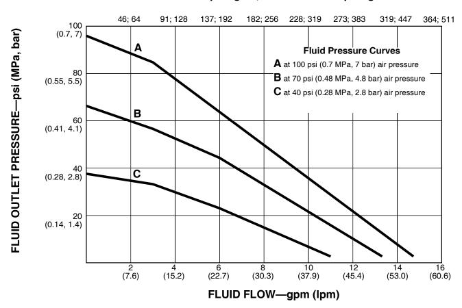
**To find Fluid Outlet Pressure** (psi/MPa/bar) at a specific fluid flow (gmp/lpm) and operating air pressure (psi/MPa/bar):
