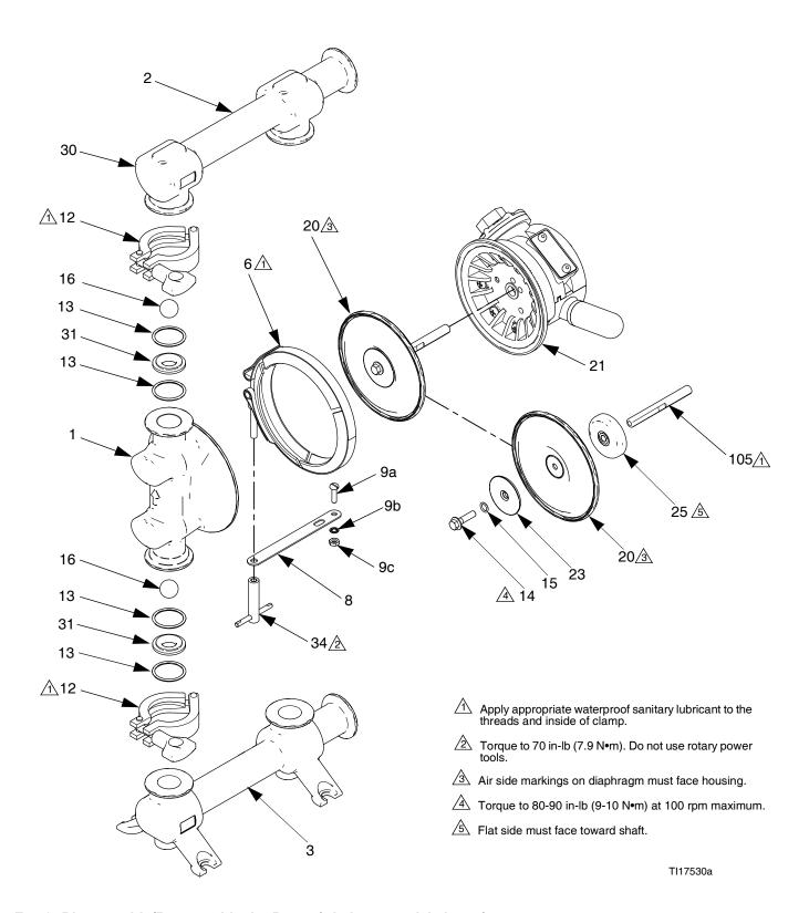
Fig. 6: Disassemble/Reassemble the Pump (tri-clamp model shown)
