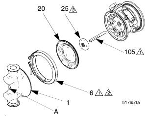
Apply appropriate waterproof sanitary lubricant to the threads and inside of clamp.
