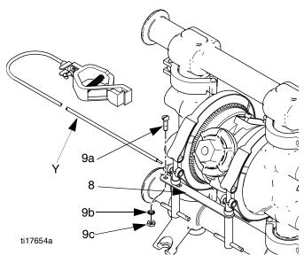
Fig. 1: Ground the pump
